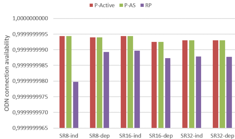
Figure 4.11.: Average ODN connection availability for the greenfield scenario of the protection schemes. The UP ODN connection availability is slightly more than four nines, while the protection schemes result in at least eight nines availability.
