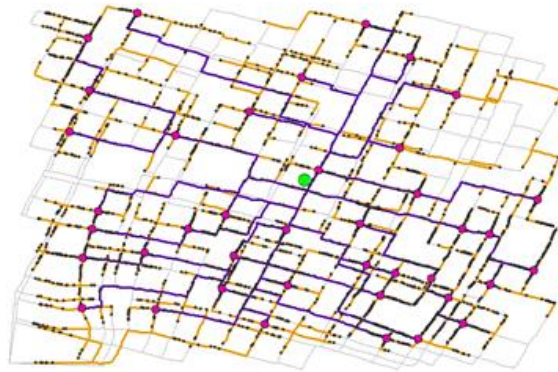
Figure 3.9.: UPON planning on the PGT-60 graph of Munich. CO is shown as green circle, remote nodes as pink circles and buildings as gray dots. The FD is shown as purple lines and the DD as orange lines.
