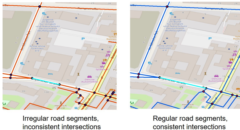
Figure A.6.: Close look on the cleaned-up line data: consistent road segments. The dangles, loops and inconsistencies were removed, the data can be used for strategic network planning.
