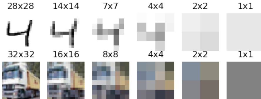
Figure 3.1: Data Hierarchy examples generated through the proposed general approach. The first row shows a sample from the MNIST dataset and the second row from the CIFAR-10 dataset. Both datasets are introduced in detail in Section 5.
