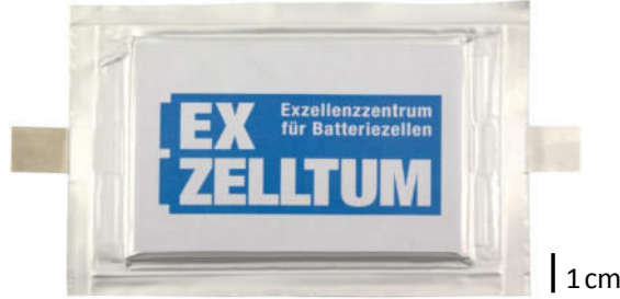
Figure 1.1.: 5 Ah pouch cell manufactured by the ExZellTUM project.
