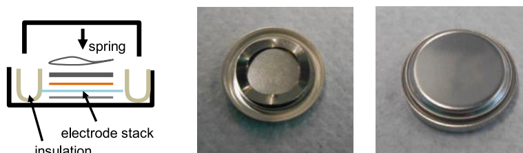
Figure 3.3.: Schematic drawing and picture of open (left) and closed (right) coin cell.
