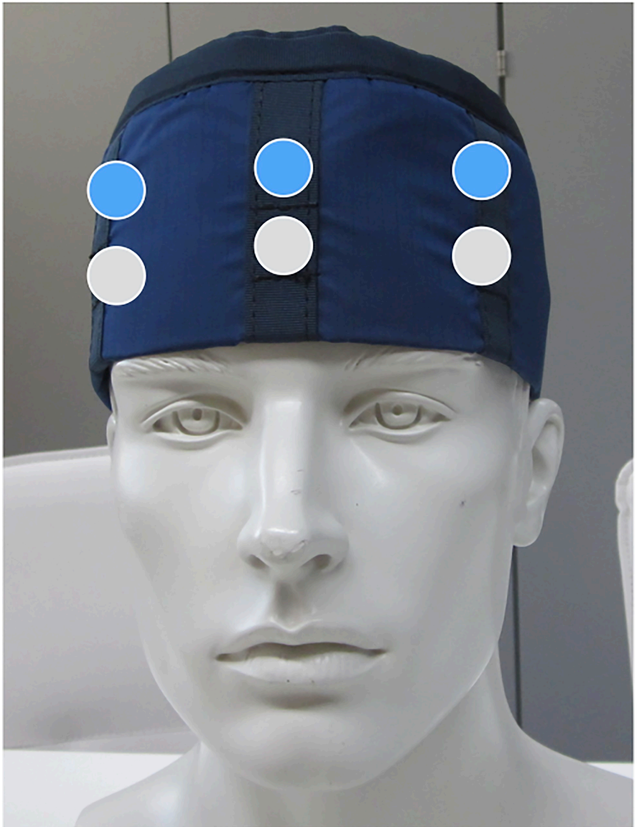
Fig 1. Position of the detectors outside (grey) and inside (blue) the cap.
