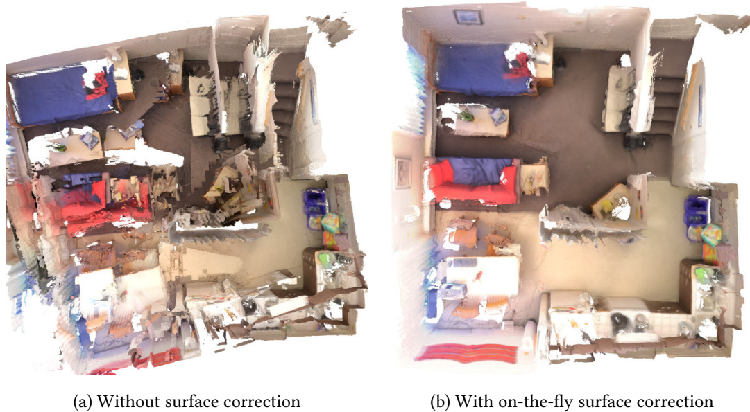
Figure 1.3: In dense real-time 3D reconstruction, RGB-D frames are immediately integrated into an SDF volume. However, the fused 3D model becomes outdated whenever camera poses are optimized for global consistency on loop closures. Without 3D surface correction, the 3D reconstruction becomes increasingly inconsistent during scanning (a). Computationally efficient methods for correcting the surface of large-scale scenes on-the-fly (e.g. Chapter 6) enable up-to-date 3D model previews in real-time (b).
