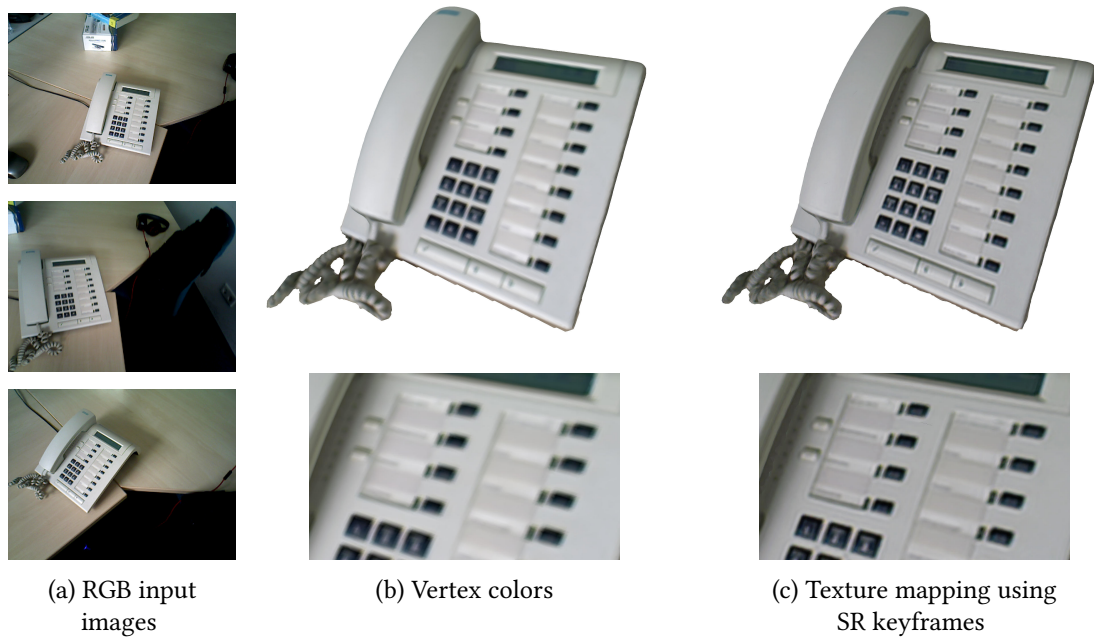
Figure 4.7: 3D model of the phone dataset reconstructed and textured using our approach: We show (a) some input images and (b) the 3D model with vertex colors only. (c) The texture mapped reconstruction provides a significantly more detailed visual appearance.
