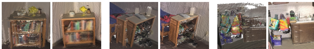
Figure 6.9: Qualitative comparison of ElasticFusion [123] (left) with our method (right) on BundleFusion/apt0 . The point cloud reconstructed with ElasticFusion exhibits artifacts due to potentially undetected loop closures and surface warping artifacts, whereas our method successfully corrects the model.
