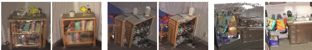
Figure 9: Qualitative comparison of ElasticFusion [21] (left) with our method (right) on BundleFusion/apt0 . The point cloud reconstructed with ElasticFusion exhibits artifacts due to potentially undetected loop closures and surface warping artifacts, whereas our method successfully corrects the model.
