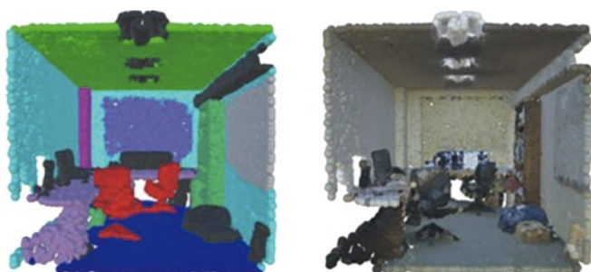
2 | Semantic segmentation (left) of a point cloud obtained by scanning an indoor environment (right) using geometric deep learning. (Figure from [2])
