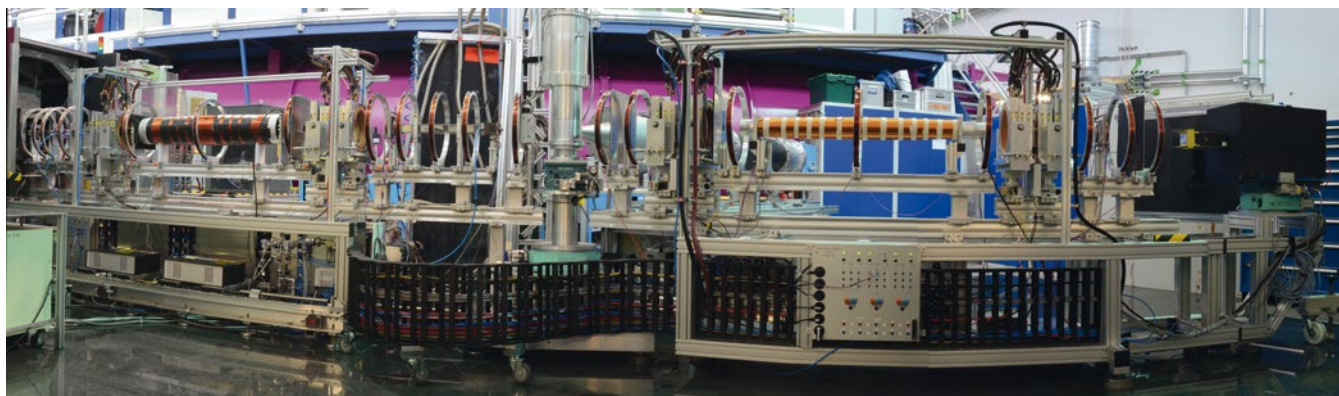
1 | (a) The Neutron Resonance Spin-Echo (NRSE) Spectrometer RESEDA at the research reactor of the Heinz Maier-Leibnitz Zentrum (MLZ).
