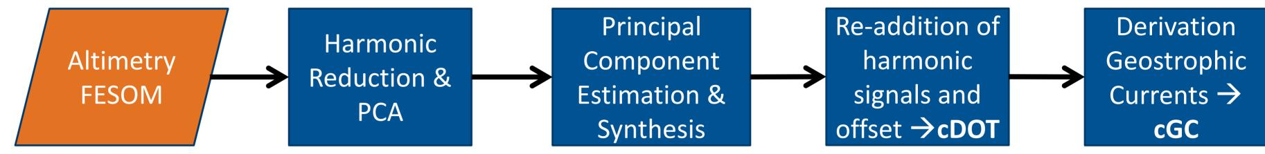
Processing scheme of combination approach based on along-track altimetry observations and FESOM modeled water heights
