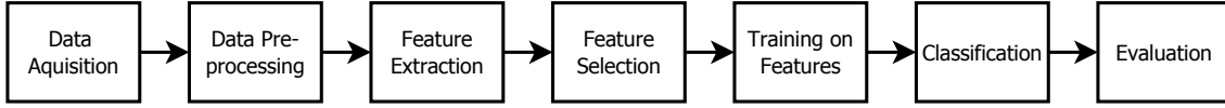
Figure 7.1.1: The architecture of a classical machine learning approach always requires domain specific expert knowledge for finding types of features with class-discriminative potential in the hand-crafted feature extraction process step three.
