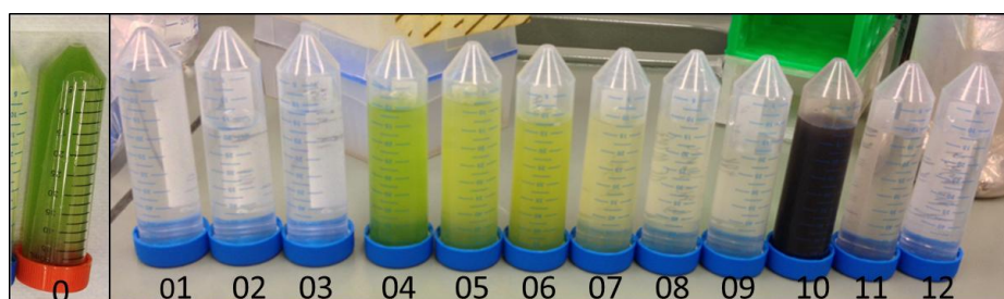
Figure 7. Fractions of the HGMS process with 5 L microalgae suspension, 0.5 \text{ g}_{\text{BION}}/\text{g}_{\text{microalgae}} , pH 6.75. Fraction 0 shows the native algae suspension (initial situation); fraction 01 corresponds to the separation step and includes the BG-11 medium; fraction 02 and 03 were collected after washing and are mainly residual salts in water; fractions 04 to 09 were collected during the microalgae recovery steps and contain only microalgae and water; fractions 10 to 12 were collected during the BIONs resuspension step and correspond to the recovery of the nanoparticles.
