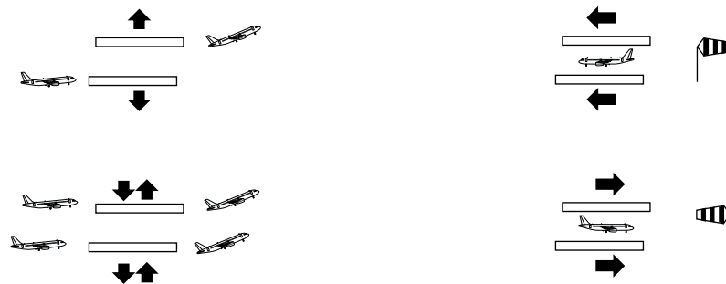
Fig. 3-9 Different airport runway usages: On the left arrivals and departures separated (top) versus mixed-mode (bottom). On the right western versus eastern operation.
