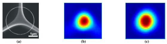
**Fig. 1** (a) SEM of the air-suspended solid-core PCF with core diameter of  $1 \mu m$ . The dashed circle indicates the approximate size of the directly coupled VCSEL with aperture size of 5  $\mu m$ . (b) Measured mode intensity profile at the output of the fiber for 1674 nm and (c) for 2004 nm, recorded by a CCD camera. The scale of (b) and (c) is roughly equal to the scale of SEM plot.
