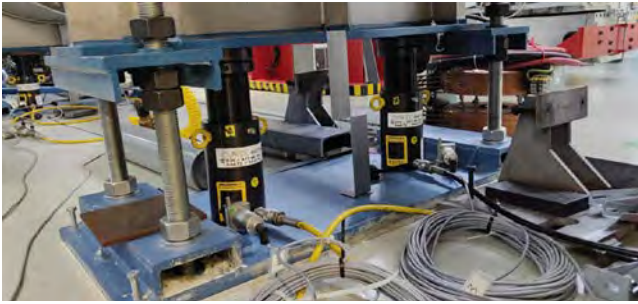
Figure 5: Hydraulic posts were used to carefully lift the KWS-2 detector tube.
