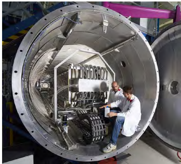
Alfonso Chacon (left) and Dr. Sebastian Mühlbauer (right) adjust the detector of the small angle neutron scattering instrument SANS-1.
