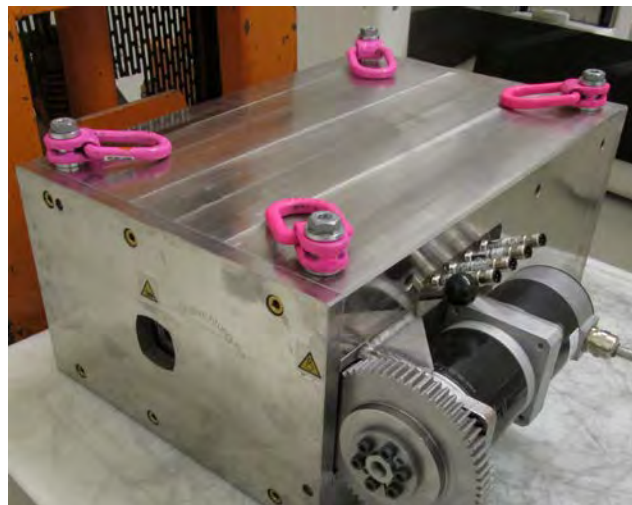
Figure 2: Collimator, ready for installation in the filter chamber, the so-called "Beckenwandnische".
