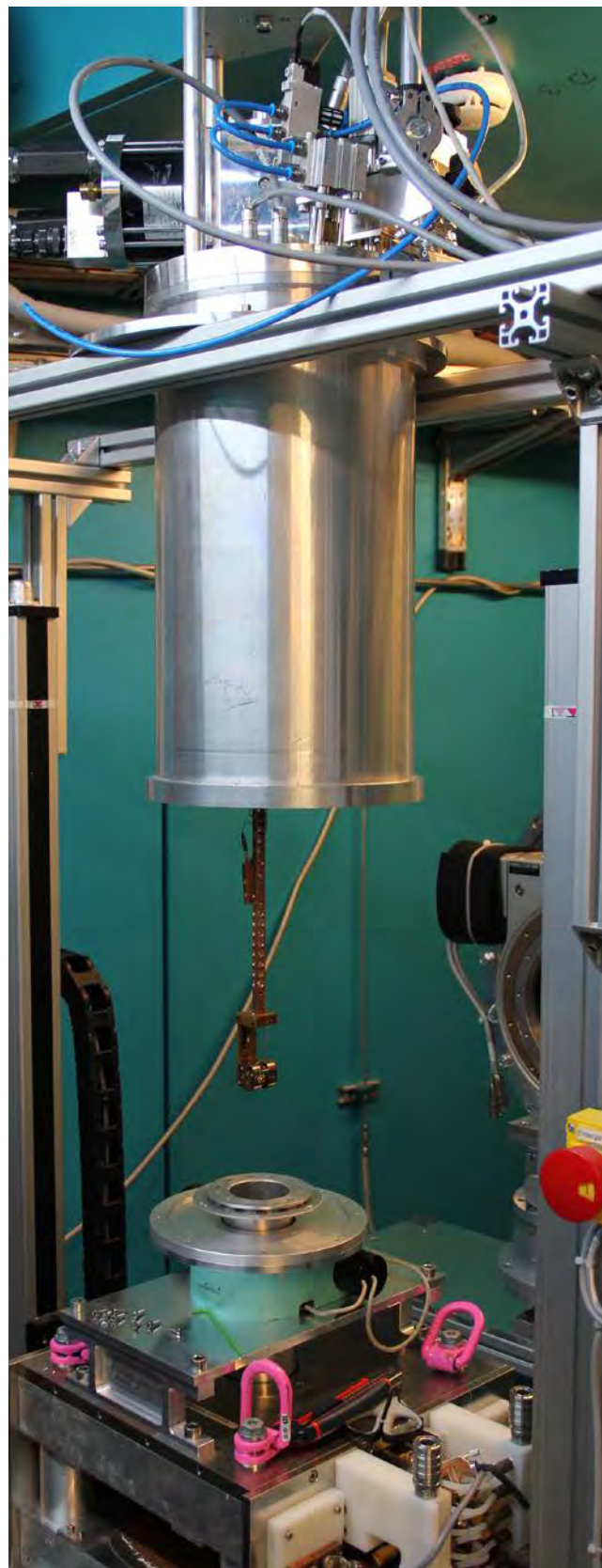
Figure 1: The new 3 He bottom-loader cryostat in the sample change position at ANTARES. For a test of the cooling performance, a pressure cell was mounted on the sample holder.
