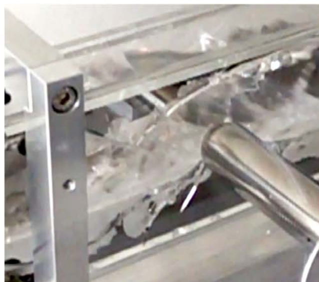
Figure 6: On the right-hand side standard neutron guide element with provoked implosion, on the left-hand side laminated glass guide element under equivalent conditions.
