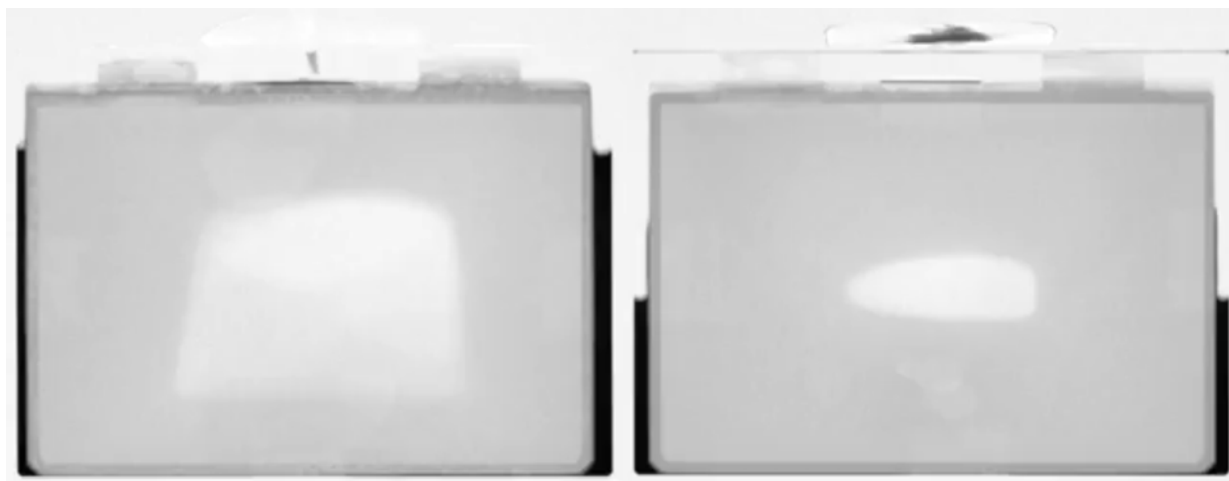
Figure 2: The tomography shows the difference between the electrode wetting at atmospheric pressure (left) and in a vacuum (right). A vacuum accelerates the wetting process by a factor of 2. The wetting of the electrode (dark area) proceeds evenly from all sides.
