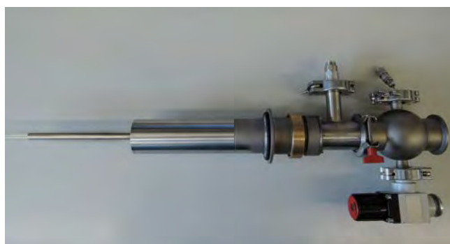
Figure 1: a) gas center stick and b) its modular setup
