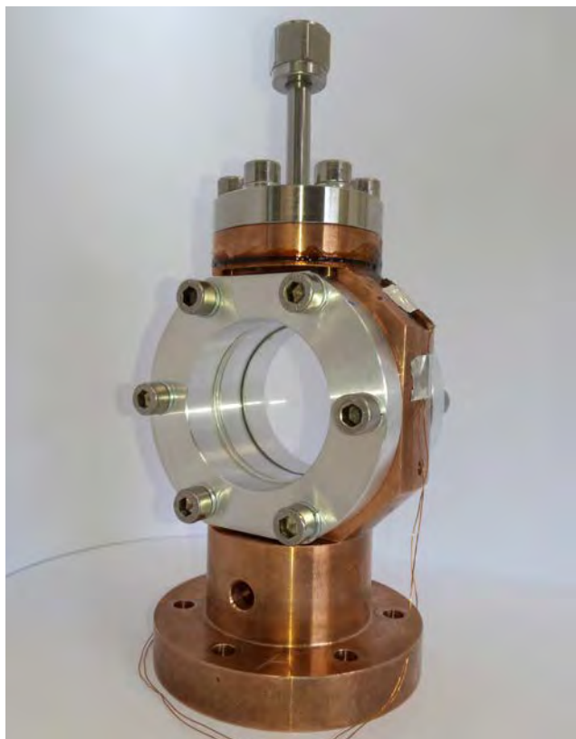
Figure 1: Sample container for cryogenic liquids and solids featuring highly polished and transparent windows.
