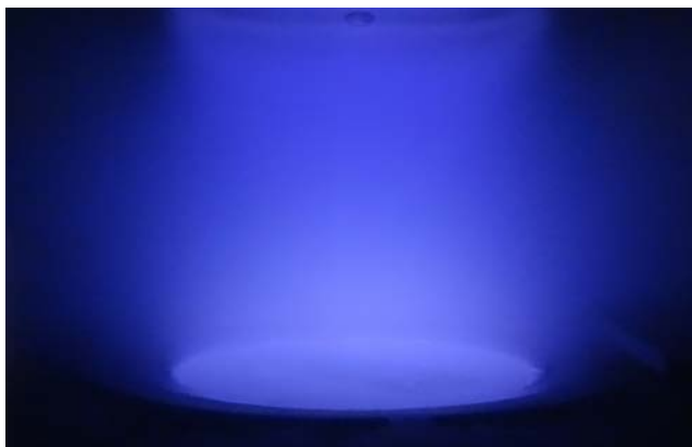
Figure 3: Burning plasma during the cleaning process of the uranium foil prior to coating.
