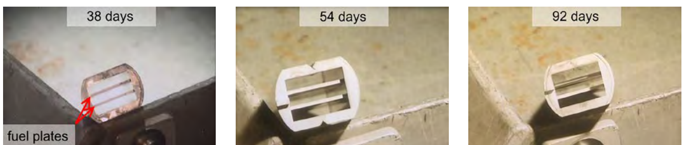
Figure 1: EMPIrE irradiation capsule with fuel plates after irradiation for 38, 54 and 92 days, respectively.
