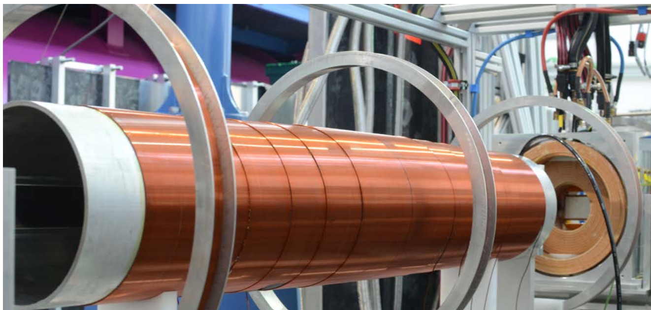
Figure 4: Conventional air-cooled solenoid as a field subtraction coil surrounded by two longitudinal guide field coils on the primary spectrometer arm of RESEDA. The second longitudinal radio-frequency (rf) flipper is shown on the right-hand side.
