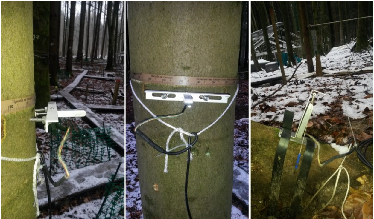
Fig 11 Automatic radius dendrometer of the DR type (Ecomatik, Dachau, Germany) in breast height and of the DC2 type on the main root of a experimental tree.
