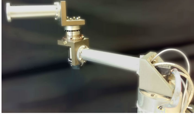
Fig. 2: Two-DOF serial robot used in experiments.
