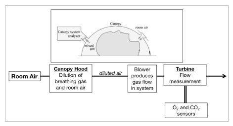
Figure 4: The principle of indirect calorimetry (according to Cosmed s.r.l., Rome, Italy). O<sub>2</sub>, oxygen; CO<sub>2</sub>, carbon dioxide.
