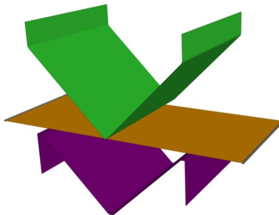
**Fig. 4-28. Simulation model of the radius forming setup**
