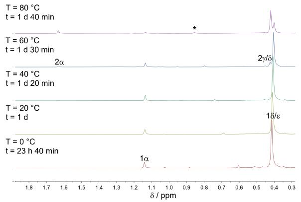
Figure S47. Temperature-resolved <sup>1</sup>H NMR study of the reaction solution of K[Ge<sub>3</sub>[Si(SiMe<sub>3</sub>)<sub>3</sub>]<sub>3</sub>] (30 mg, 0.021 mmol) and pivaloyl chloride (2.6  $\mu$ L, 0.021 mmol) in 0.6 mL [D8]toluene after reaction time t. The compounds were first reacted at 0 °C for 23 h and 40 min before the <sup>1</sup>H NMR spectrum at 0 °C was recorded. The temperature was then slowly raised. Signals marked with \* could not be assigned.
