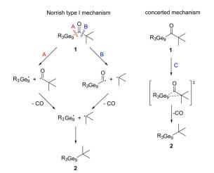
Scheme 2. Three conceivable reaction pathways of the decarbonylation of 1 yielding 2. Reaction pathways A and B follow a Norrish-type I  $\alpha$ -bond cleavage. Reaction pathway C runs through a concerted transition state.
