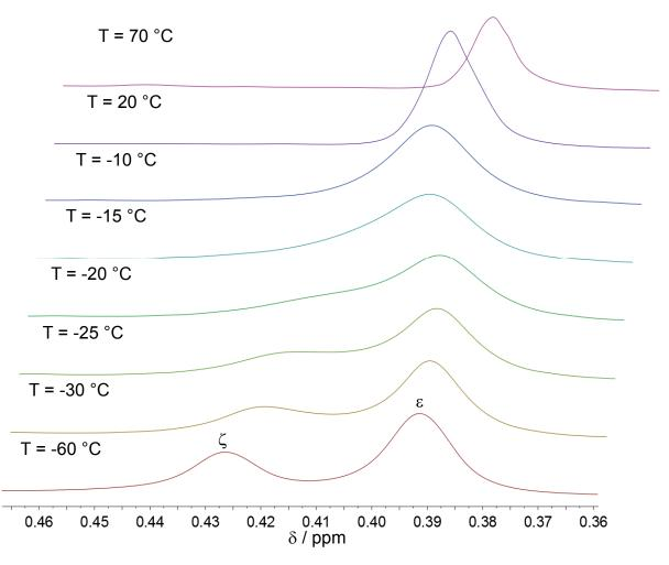
According to the temperature-dependent <sup>1</sup>H NMR spectra in figure S14 the coalescence temperature T<sub>c</sub> is regarded to be 258 K. Assuming that the rotation obeys the rate law of a first order reaction the rate constant of the rotation  $k_r$  at T<sub>c</sub> according to Eyring equation is 31.1 s<sup>-1</sup>. Therefore the Free Gibbs Energy of the rotation ( $\Delta G_{258}$ ) is determined to be 55.4 kJ mol<sup>-1</sup>.
