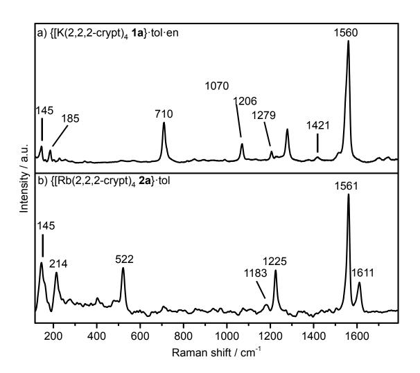
The signals at 145 and 185 cm<sup>-1</sup> for **1a** and at 145 and 214 cm<sup>-1</sup> for **2a** are in the range of the skeletal vibrations of bare Ge<sub>9</sub> clusters.<sup>5</sup> The band at 522 cm<sup>-1</sup> is indicative of the *exo*-Ge-C
