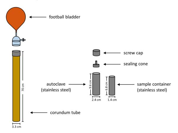
Figure 2.1.1. Corundum tube and stainless steel autoclave used for the synthesis of K<sub>4</sub>Ge<sub>9</sub>.
