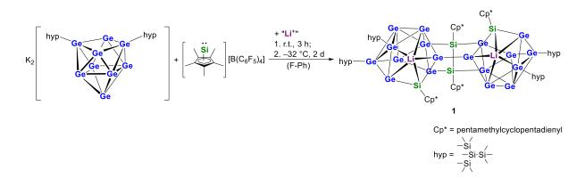
**Scheme 1.** Reaction of  $K_2[{(Me_3Si)_3Si}_3Ge_9]$  with  $[SiCp^*][B(C_6F_5)_4]$  in the presence of Li cations yielding **1**.
