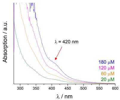
**Figure S15.** UV-Vis electronic spectrum of [K(2,2,2-crypt)][{(Me<sub>3</sub>Si)<sub>3</sub>Si}<sub>3</sub>Ge<sub>9</sub>] (7) in toluene ( $\lambda$  = 280 – 600 nm, c<sub>M</sub> = 20 –180 µM).
