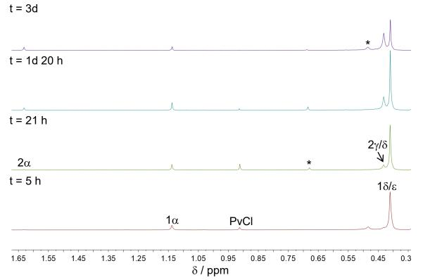
Figure S43. Time-resolved <sup>1</sup>H NMR study of the reaction solution of K[Ge<sub>9</sub>{Si(SiMe<sub>3</sub>)<sub>3</sub>}] (30 mg, 0.021 mmol) and pivaloyl chloride (2.6 µL, 0.021 mmol) in 0.6 mL [D8]toluene at r.t. after reaction time t under exclusion of light. Signals marked with \* could not be assigned.
