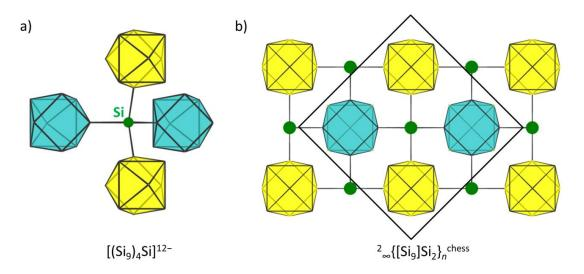
**Figure 2.** Schematic presentation of interconnected clusters in a) predicted  $[(Si_9)_4Si]^{12-[36]}$  and b) predicted  $\overset{2}{_{\sim}}{[Si_9]Si_2}_n^{chess}$ . The different colors indicate different orientations.
