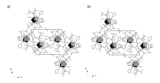
**Figure S1.** Illustration of the unit cells of a) **1** and b) **2**. [*M*Ge<sub>9</sub>] cluster cores (M = Ni, Pt) are shown as dark-grey polyhedra. Functionalities and solvent molecules are shown schematically. Hydrogen atoms are omitted for clarity.
