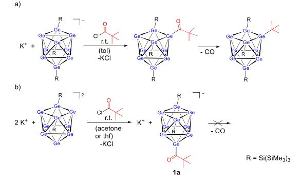
**Scheme 1.** a) Reaction of  $K[\{(Me_3Si)_3Si\}_3Ge_9]$  with pivaloyl chloride yielding  $\{(Me_3Si)_3Si\}_3Ge_9(CO)tBu$ , which in a subsequent step eliminates CO under formation of  $\{(Me_3Si)_3Si\}_3Ge_9tBu$ . b) Reaction of  $K_2[\{(Me_3Si)_3Si\}_2Ge_9]$  with pivaloyl chloride yielding  $K[\{(Me_3Si)_3Si\}_2Ge_9(CO)tBu]$ , which does not eliminate CO. R depicts the hypersilyl ligands.
