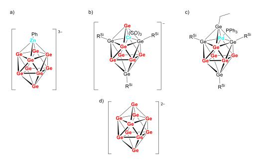
**Figure 3.4.2.** Structure of a)  $closo-[Ge_9ZnPh]^{3-},^{[17]}$  b)  $closo-[{(Me_3Si)_3Si}_3Ge_9Cr(CO)_3]^{-},^{[20]}$  c)  $closo-[{(Me_3Si)_3Si}_3EtGe_9Pd(PPh_3)]$ , and d)  $closo-[Ge_{10}]^{2-},^{[22]}$  The unsubstituted, "naked" vertices are highlighted in red. R<sup>Si</sup> depicts the tris(trimethylsilyl)silyl ligands attached to the cluster core.
