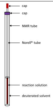
Figure 2.2.1. NMR setup for *in situ* investigations of reactions carried out in non-deuterated solvents.
