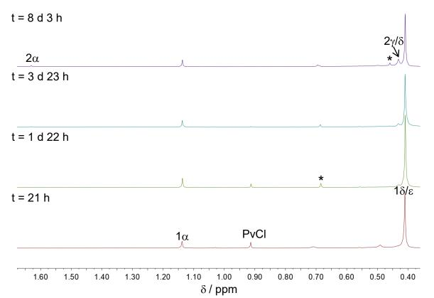
Figure S46. Time-resolved <sup>1</sup>H NMR study of the reaction solution of K[Ge<sub>3</sub>{Si(SiMe<sub>3</sub>)<sub>3</sub>]<sub>3</sub>] (30 mg, 0.021 mmol) and pivaloyl chloride (2.6  $\mu$ L, 0.021 mmol) in 0.6 mL [D8]toluene at 2 °C after reaction time t. Signals marked with \* could not be assigned.
