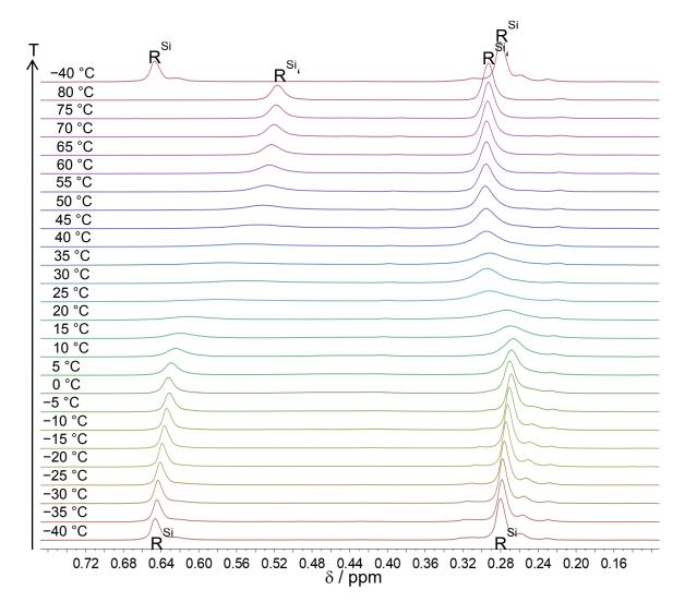
**Figure 3.4.4.** Stacked excerpt of the relevant section of the temperature-dependent <sup>1</sup>H NMR spectra of **37** recorded in  $[D_8]$ toluene. R<sup>Si</sup> depicts the silyl ligands of **37** and R<sup>Si</sup> the silyl ligands of the high-temperature-isomer of **37**. The figure was modified on the basis of ref. [25].
