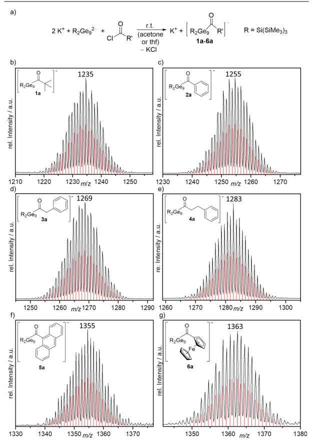
**Figure 1.** a) Reaction of  $K_2[Ge_9{Si(SiMe_3)_3}_2]$  with Cl(CO)R' yielding the anions **1a-6a**. b)-g) ESI mass spectra of the anions **1a-6a** recorded in thf-reaction solutions in the negative ion mode. The measured spectra are shown in black and the corresponding simulated patterns are shown as bar graphs below. R represents the hypersilyl ligands.
