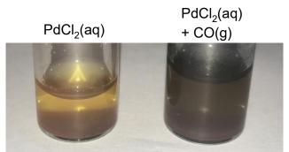
Figure S48. CO detection reaction with a saturated aqueous solution of PdCl<sub>2</sub>. The gas phase of a reaction solution after almost complete conversion of 1 into 2 (see Figure S49) was injected into a saturated, pale orange aqueous solution of PdCl<sub>2</sub>. Elemental Pd occurs after 2 minutes and appears as metallic precipitate.
