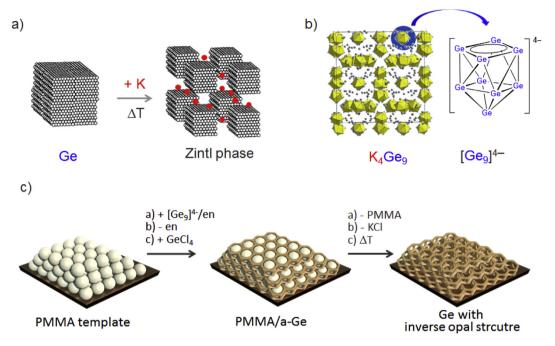
**Fig. 1.** Formation of a Zintl phase by the reaction of an alkali metal element with a p-block (semi)metal. (b) The Zintl phase  $K_4Ge_9$  comprises discrete  $[Ge_9]^{4-}$  cluster anions. (c) Formation of elemental germanium with a novel morphology. Impregnating a PMMA template structure with a  $[Ge_9]^{4-}$ /en solution, cluster linking/oxidation with GeCl<sub>4</sub>, and removal of KCl and PMMA results in mesostructured Ge. PMMA, polymethylmethacrylate; en, ethylenediamine.
