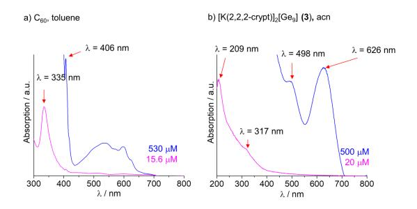
**Figure 3.1.2.** UV-Vis electronic spectra of a)  $C_{60}$  in toluene at concentrations of 530 and 15.6  $\mu$ M in the region of 300 to 800 nm and of b)  $[K(2,2,2-crypt)]_2[Ge_9]$  (**3**) in acetonitrile (acn) at concentrations of 500 and 20  $\mu$ M in the region of 200 to 800 nm. The figure was modified on the basis of ref. [21].
