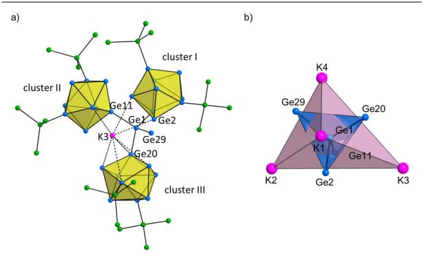
**Figure 3.** a) Excerpt of the structure of **1**. The Ge<sub>9</sub> clusters are shown as yellow polyhedra. The methyl groups of the silyl ligands are omitted for clarity. b) Interpenetrating tetrahedrons formed by the coordinated potassium cations (depicted in purple) and the germanium atoms bound to the central Ge1 (depicted in blue). All atoms are shown as spheres. Color code: Ge – blue, Si – green, K – pink.
