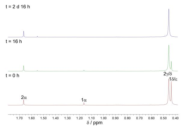
Figure S44. Time-resolved <sup>1</sup>H NMR study in [D6]benzene of the dissolved residue of the reaction of 1 eq. of K[Ge<sub>9</sub>{Si(SiMe<sub>3</sub>)<sub>3</sub>]<sub>3</sub>] with 1 eq. of pivaloyl chloride in hexane after a reaction time of 17 h at r.t. and after evaporation of hexane to dryness. t abbreviates the period after redissolving of products 1 and 2 in [D6]benzene.
