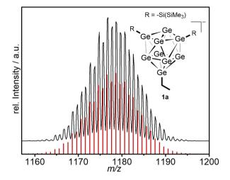
**Fig. 2.** ESI mass spectrum of a THF solution of **1** and predicted structure of **1a**. The measured spectrum of  $[CH_3CH_2Ge_3[Si(SiMe_3)_3]_2]^-$  (**1a**) is shown in black. The simulated spectrum is shown as bar graph in red. (For further information see Fig. S2 of Supporting information).
