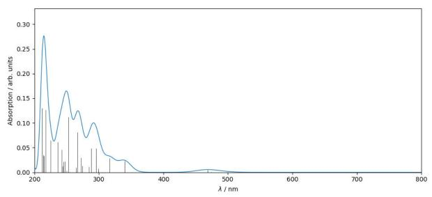
**Figure S16.** Simulated UV-Vis spectrum of  $[Ge_9]^{2-}$  in the range 200–800 nm. The black peaks are the raw data, the blue curve has been obtained from the peak data by applying Gaussian broadening of 0.25 eV.
