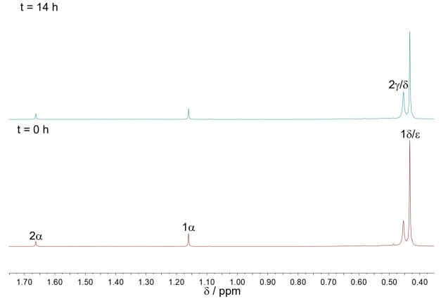
**Figure S45.** Time-resolved <sup>1</sup>H NMR study in [D6]benzene of the dissolved residue of the reaction of K[Ge<sub>3</sub>{Si(SiMe<sub>3</sub>)<sub>3</sub>}] (60 mg, 0.042 mmol) with pivaloyl chloride (5.2  $\mu$ L, 0.042 mmol) in 1.2 mL benzene after a reaction time of 16 h at r.t. and after evaporation of benzene to dryness. t abbreviates the period after redissolving products 1 and 2 in [D6]benzene.
