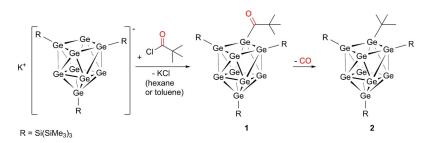
Scheme 1. Reaction of K[Ge<sub>9</sub>[Si(SiMe<sub>3</sub>)<sub>3</sub>]<sub>3</sub>] with pivaloyl chloride in hexane or toluene yielding 1. Subsequent release of CO leads to the formation of 2.
