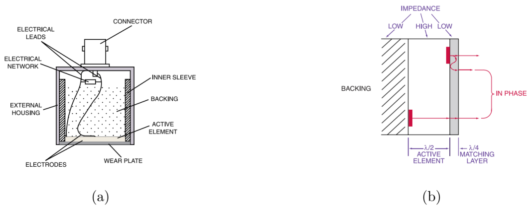
Figure 1.14: Internal configuration of piezoelectric transducer. a: After the sound is coupled into the active element, it induces an electric potential proportional to the instantaneous amplitude of the sound wave. This voltage is transported to a connector and can be measured. Finally, the sound wave is absorbed by the backing layer to avoid reflections [80]. b: Impedance matching techniques may be used to improve the coupling efficiency.
