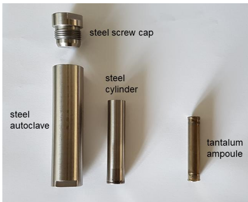
Figure 2.1: Stainless-steel autoclave and tantalum ampoule as reaction compartments for solid state reactions.
