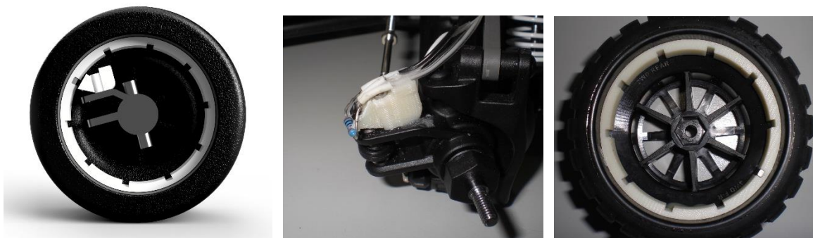
Figure 14: CAD design of sensor mount and magnet ring (left), 3D printed sensor mount (middle), 3D printed magnet ring (right)
