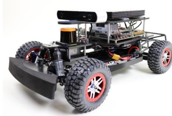
Figure 10: RACECAR/J hardware platform [59]
