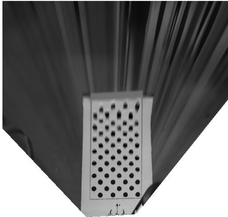
Figure 25: Image pixel transformed in world coordinates (bird's eye view)
