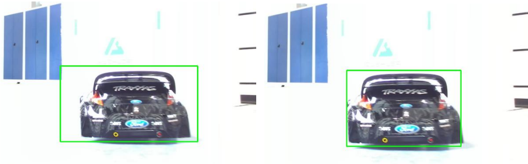
Figure 34: Detected bounding boxes using an input size of 160x160 (left) vs 640x640 (right)
