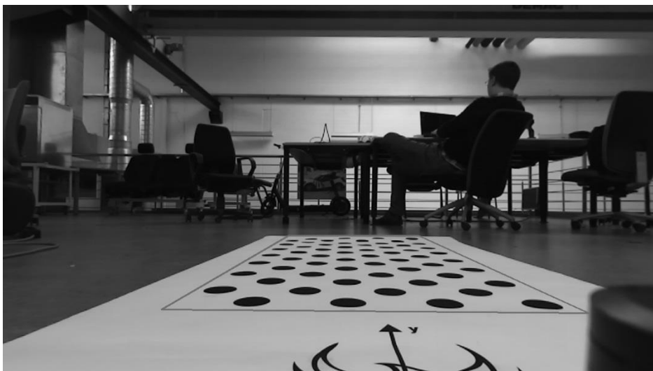
Figure 24: Rectified image showing a calibration pattern
