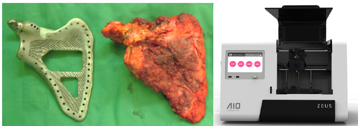
Figure 3.1.: Already existing examples for the use of RE and AM in a combined workflow. Left: prosthesis for scapula replacement, manufactured via Selective Laser Melting of titan (excised tumor displayed as well). Right: AIO Robotics ZEUS, commercial 3D-printer with replication ability [AIO Robotics, Inc. 2017; Fan et al. 2015].
