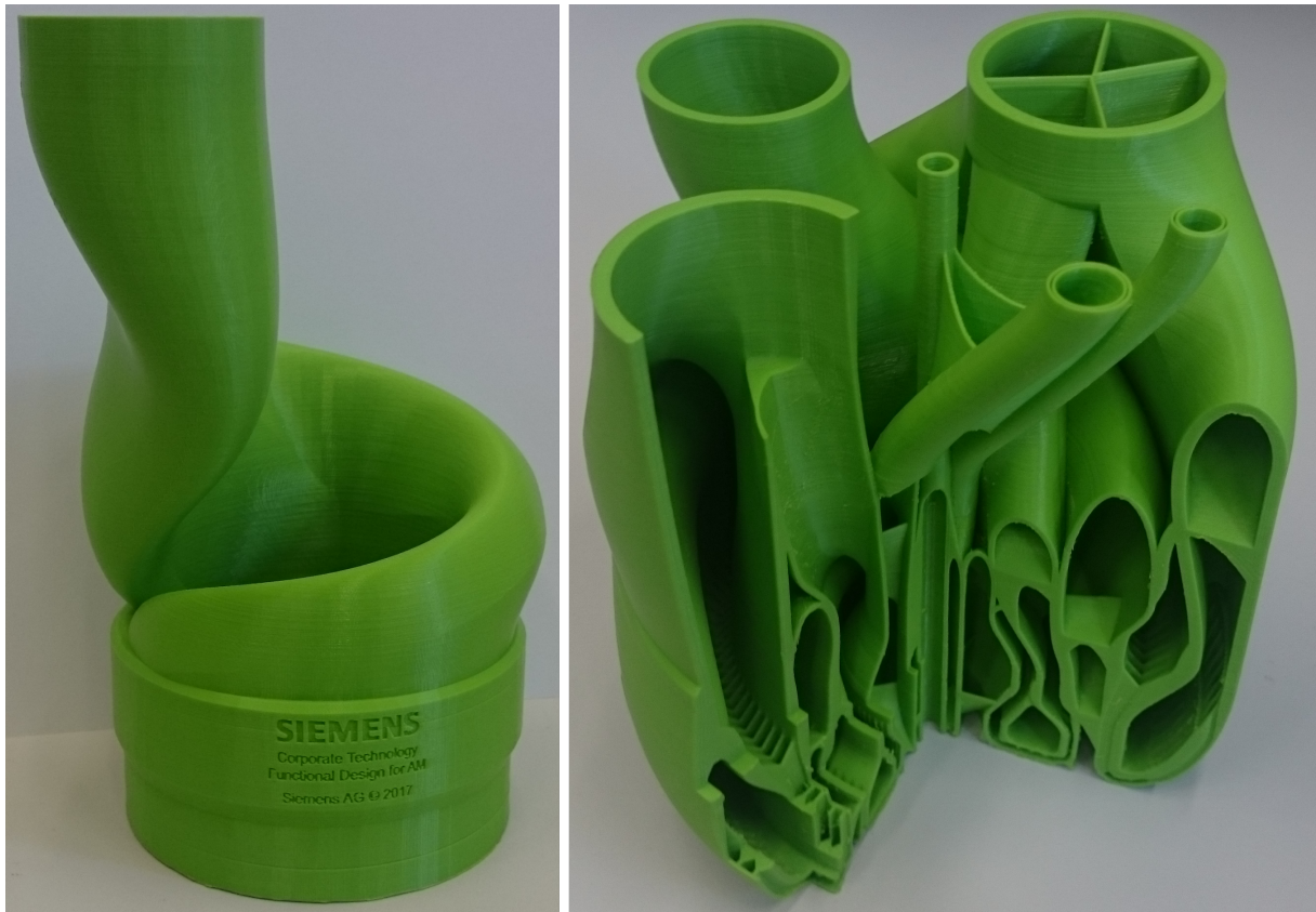
Figure 10.1.: Test pieces for our exemplary RE process. Left: a single flow swirler line, which is part of the burner tip (depicted cutted open on the right, models not to scale). The burner tip itself is highly complex and features several filigrane structures on the inside.
