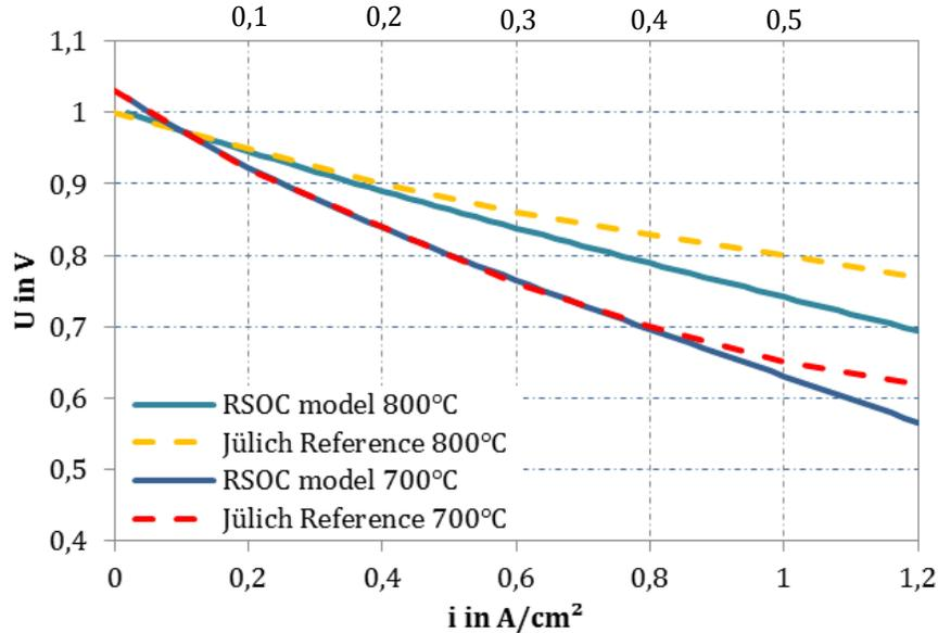
Figure 2. Comparison of the SOFC model and experimental short stack data from (5). The values shown at the upper x-axis resemble the respective fuel utilization.
