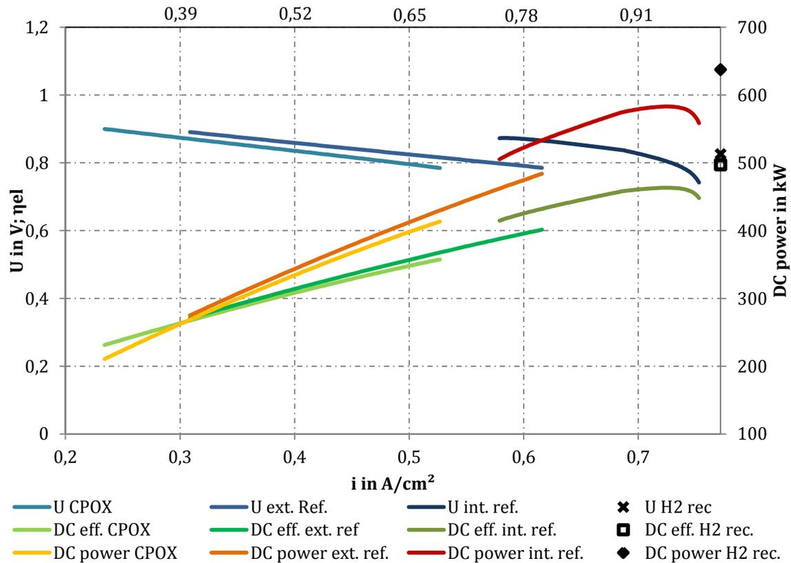
Figure 5. Results of the parameter study for SOFC operated on biogas from anaerobic digestion. The values shown at the upper x-axis resemble the global fuel utilization.
