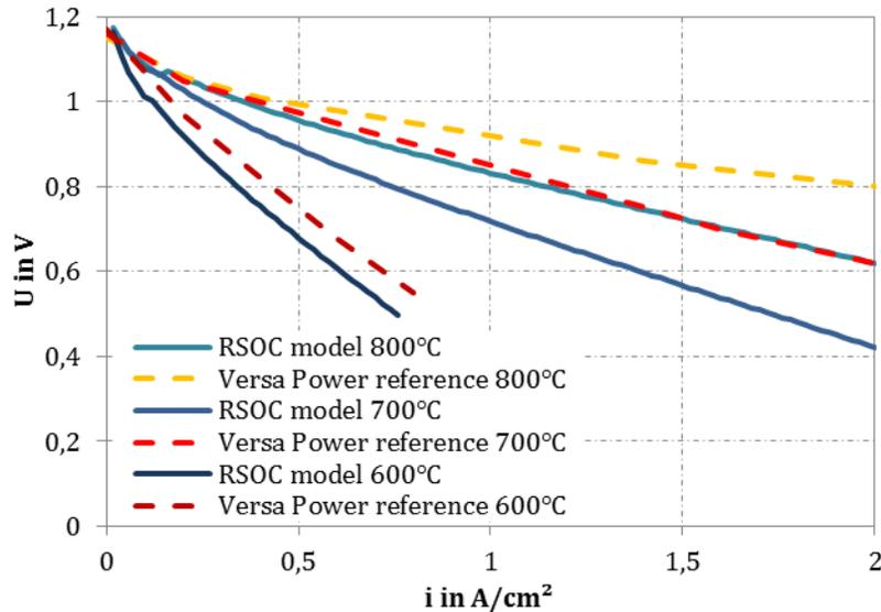
Figure 1. Comparison of the SOFC model and experimental single cell data from (4).
