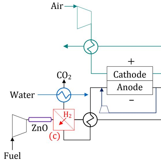
Figure 6. Simplified schematic drawing of SOFC system with water gas shift membrane and H<sub>2</sub> recovery for increased fuel utilization.
