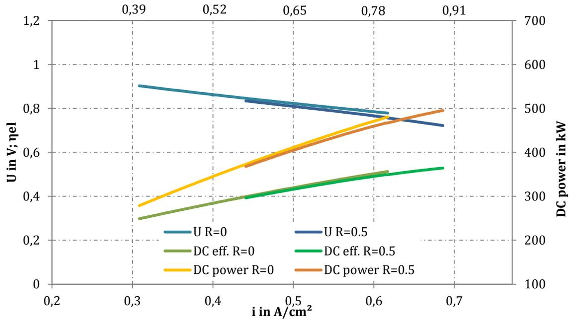
Figure 4. Results of the parameter study for SOFC operated on gasification syngas. The values shown at the upper x-axis resemble the global fuel utilization.
