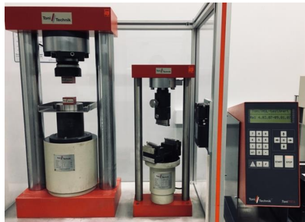
Figure 30: Test apparatus used to determine the compressive and flexural strengths of mortar
