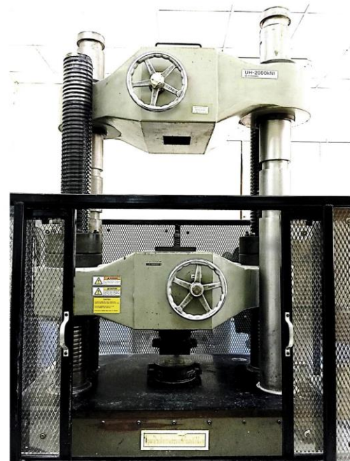
Fig. 2. Compressive strength test apparatus used in the experiments.
