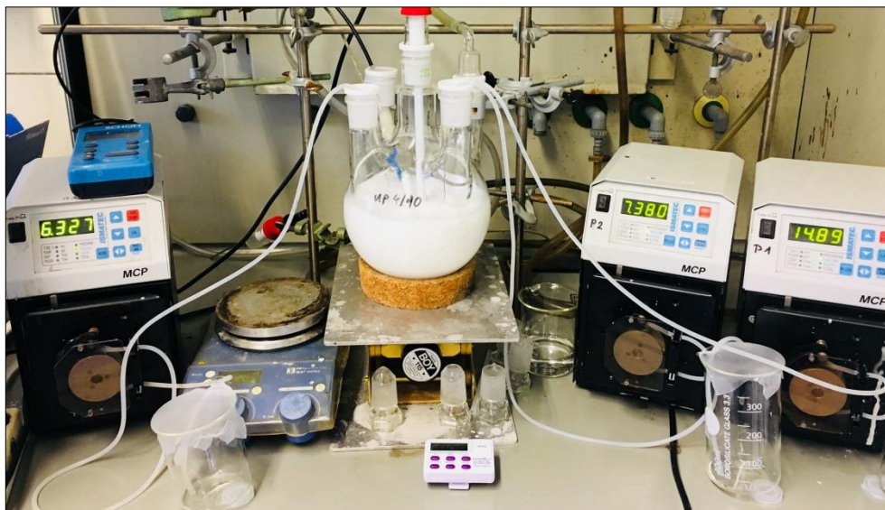
Figure 29: Experimental setup for the synthesis of the C-S-H – PCE nanocomposites
