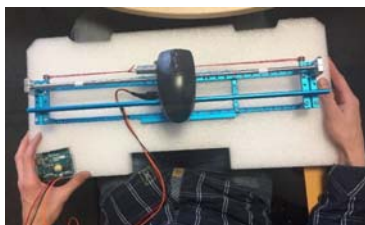
Fig. 8 Slider setup for dynamically controlling the curve depiction in the display. Participants moved the slider along the blue frame. The middle position was haptically emphasised by a resistor.
