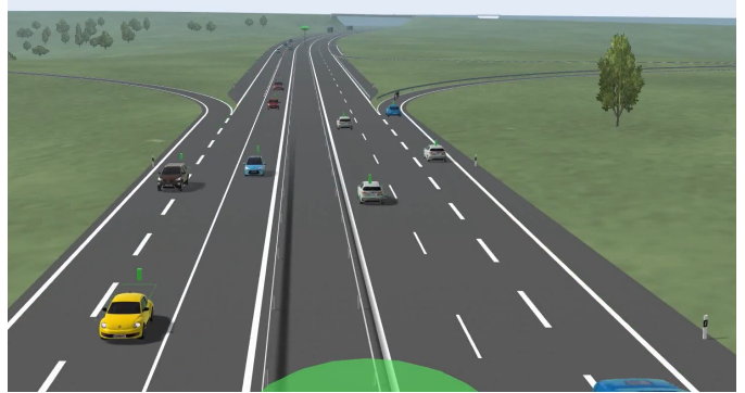
Fig. 5. The CarMaker as a dynamic virtualization platform for the real time digital twin model, showing two infrastructure measurement points in a highway scenario perceiving a number of vehicles Source: IPG CarMaker .
