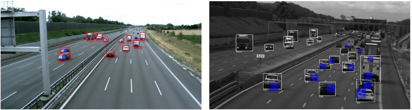
Fig. 3. View of the short-range camera on the left and of the long-range camera on the right with camera detections (bounding boxes) and radar measurements (blue cuboids). The image illustrates fields of views and detection ranges of the 2 cameras and the radar. The sensors complement each other. The short-range camera detects objects closer than the radar, the far range camera detects objects beyond the radar range. There is overlap between each sensor.
