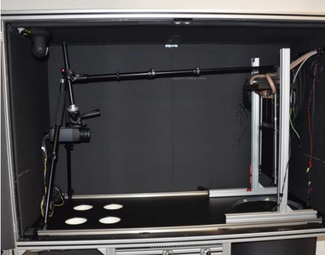
Figure 3.2: Picture of a thermal camera setup to measure the surface temperature of a pouch cell [106]
