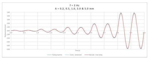
Fig. 5 Resulting amplitudes of five different experiments (1 sec period each experiment)
