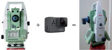
Fig. 1 IATS prototype: Leica TPS1201 & GoPro5 Hero camera
