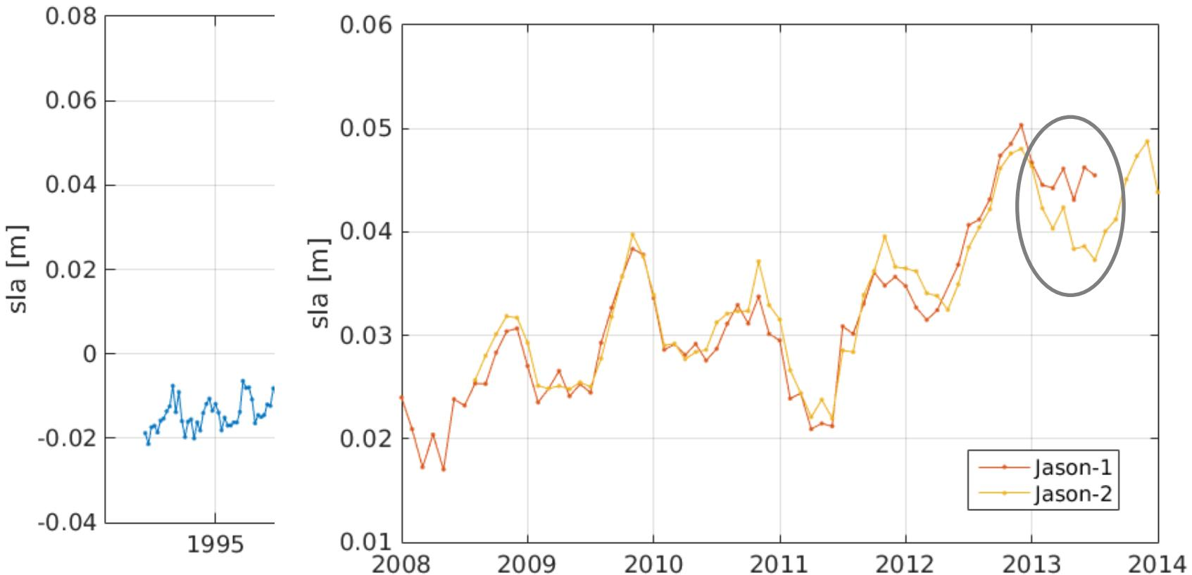
⇒ Significant discrepancies remain after removing a constant offset
