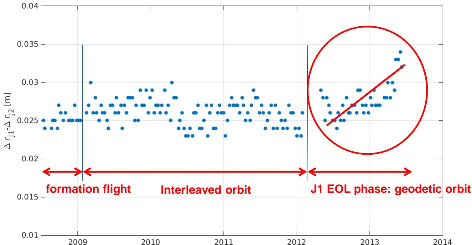
=> drift in radial errors (Jason-1 EOL)
