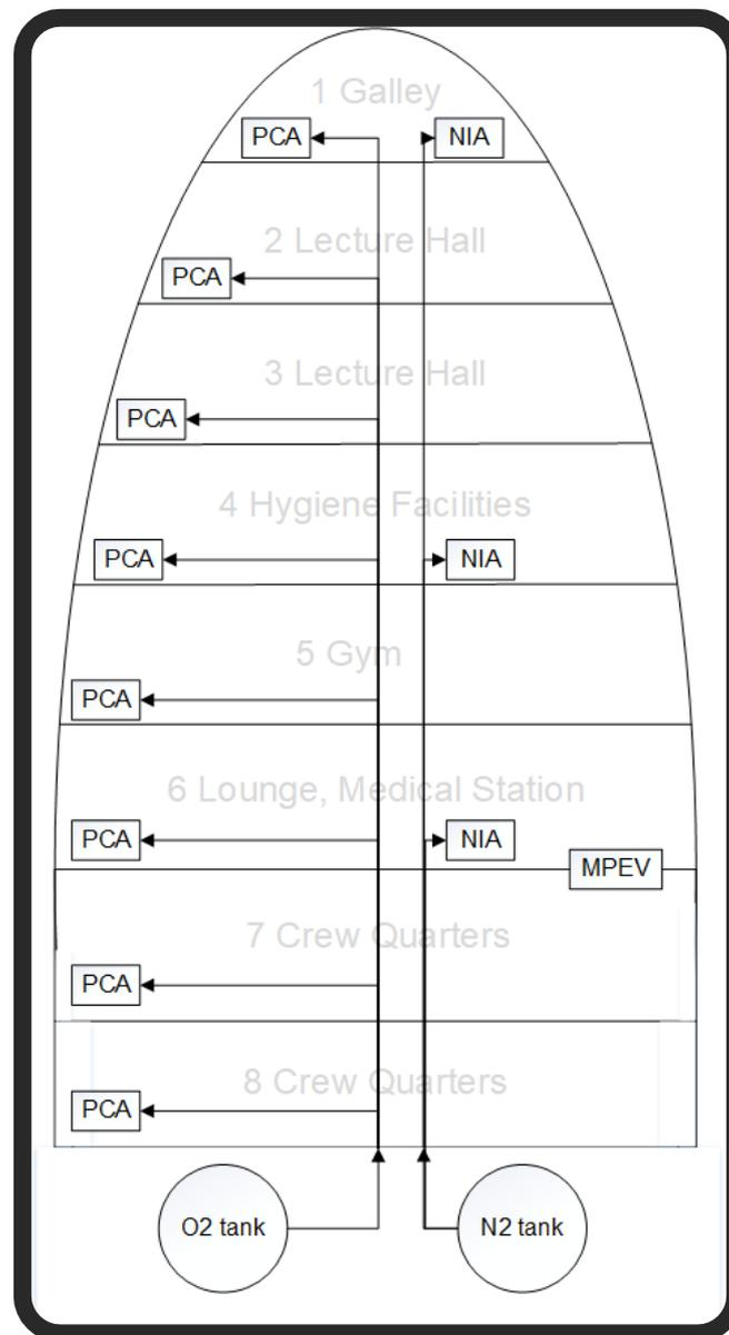
Figure 10-1: Schematic of the ACS system
