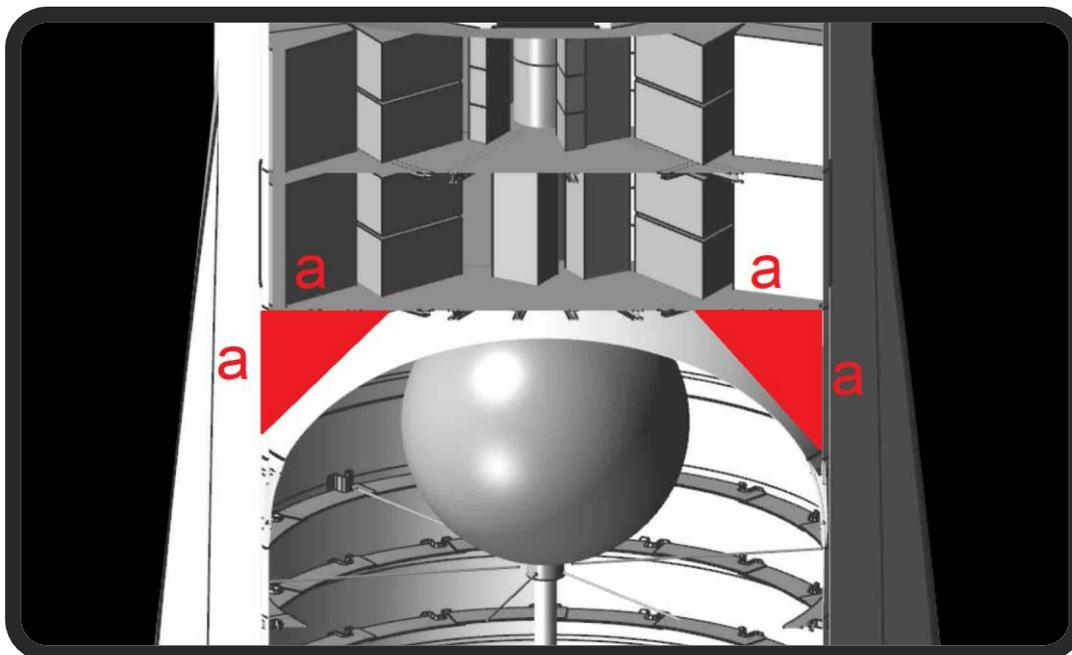
Figure 6-4: Unpressurized space between lowest deck and propellant tank [11]
