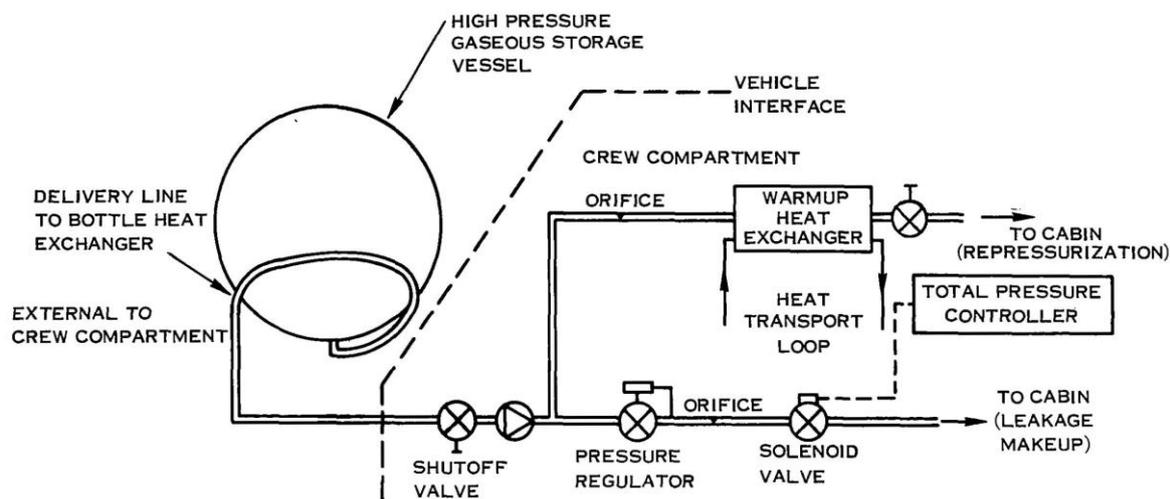
Figure 6-3: High pressure gaseous storage concept [50, p. 75]
