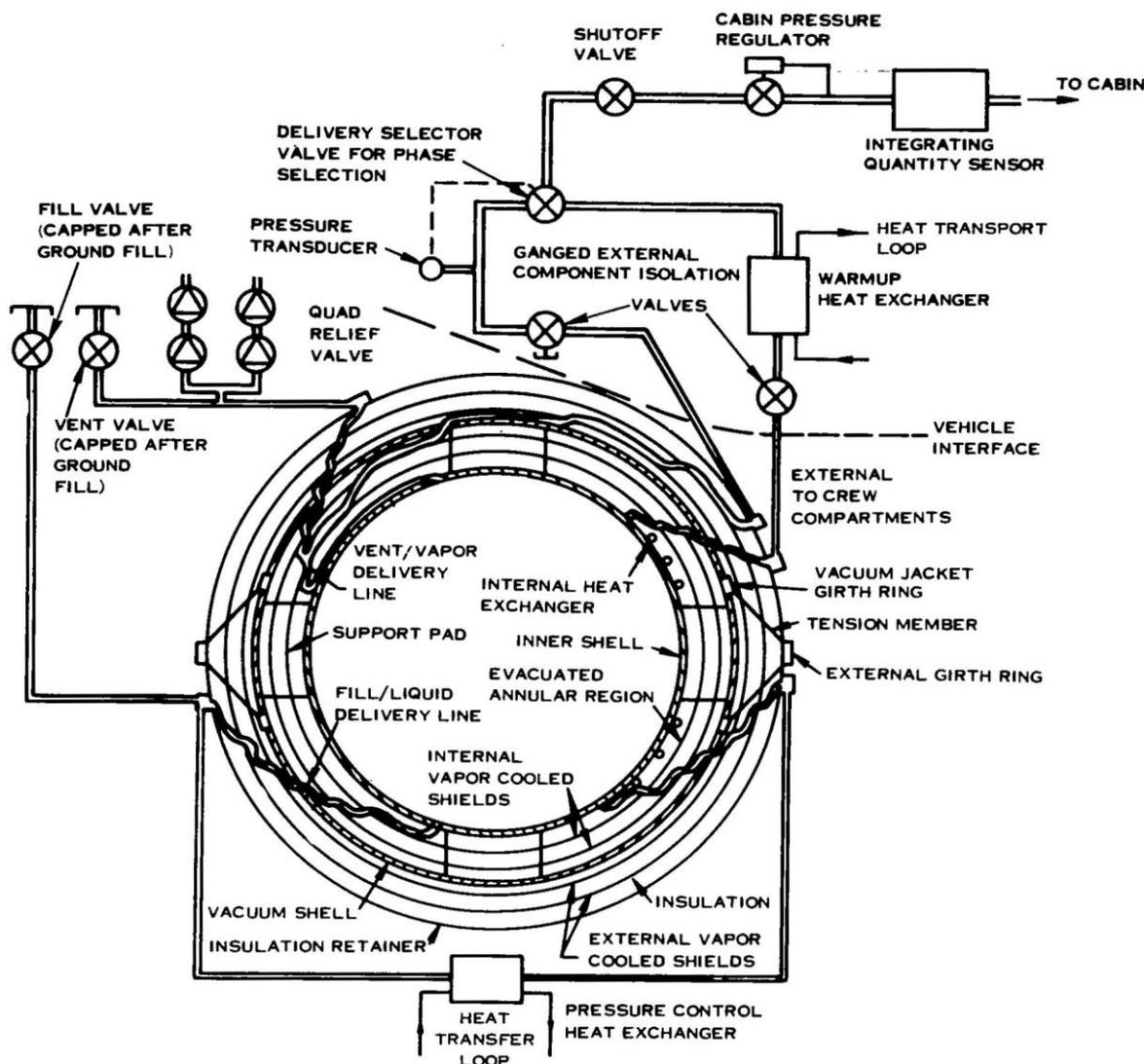
Figure 6-5: Cryogenic storage system schematic [50, p. 97]
