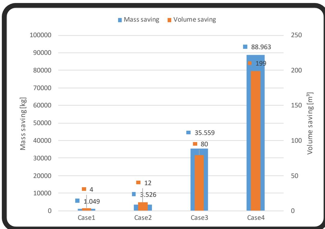
Figure 10-19: Mass and volume savings of the considered trade cases in comparison to a baseline storage system
