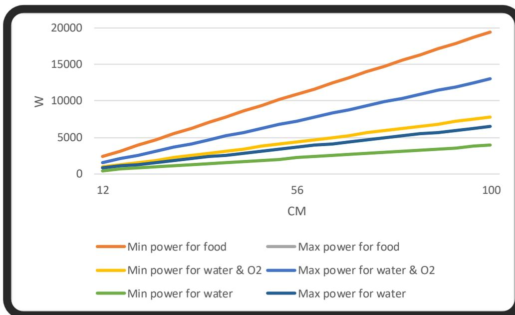
Figure 9-4: Required power for plant growth
