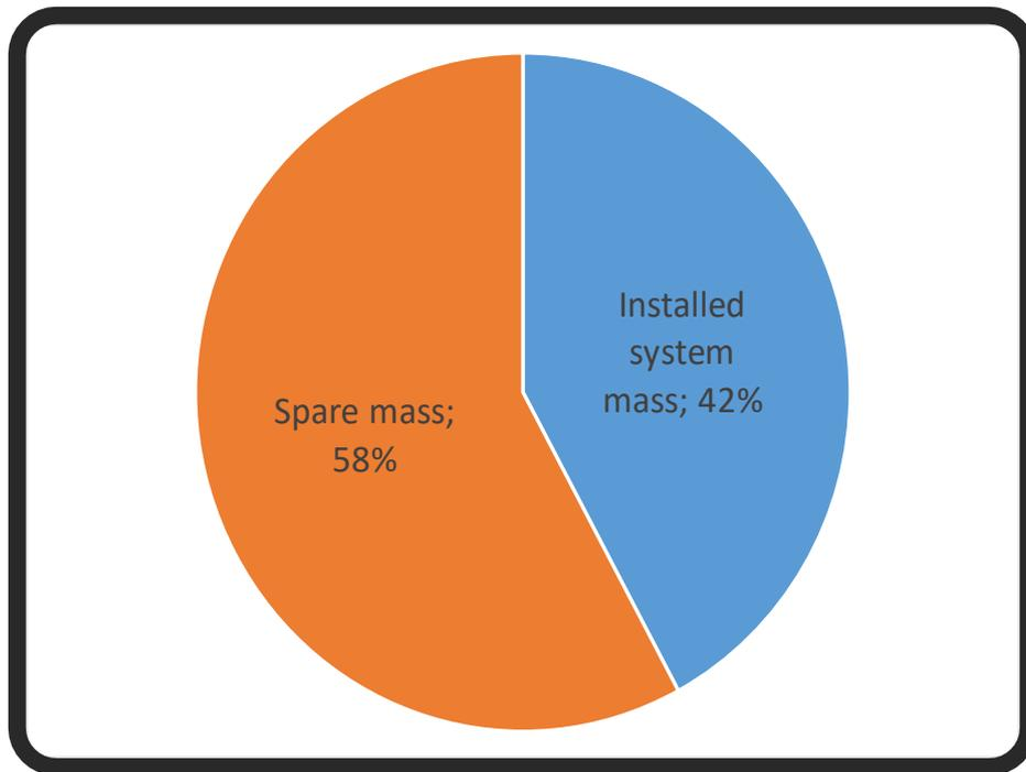
Figure 9-5: Contingent of spare mass for the water recovery system
