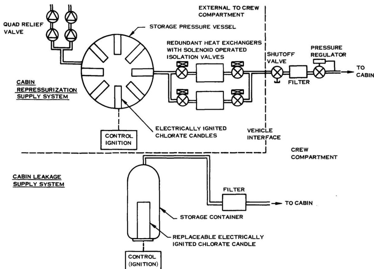
Figure 6-6: Oxygen candle system schematic [50, p. 79]
