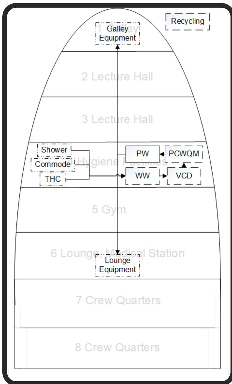
Figure 10-17: Schematic of the final WRM design
