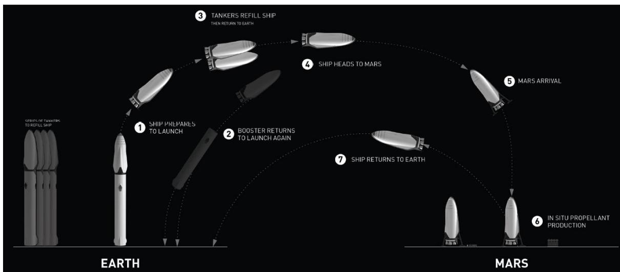
Figure 3-1: Proposed high-level operations profile by SpaceX [1]
