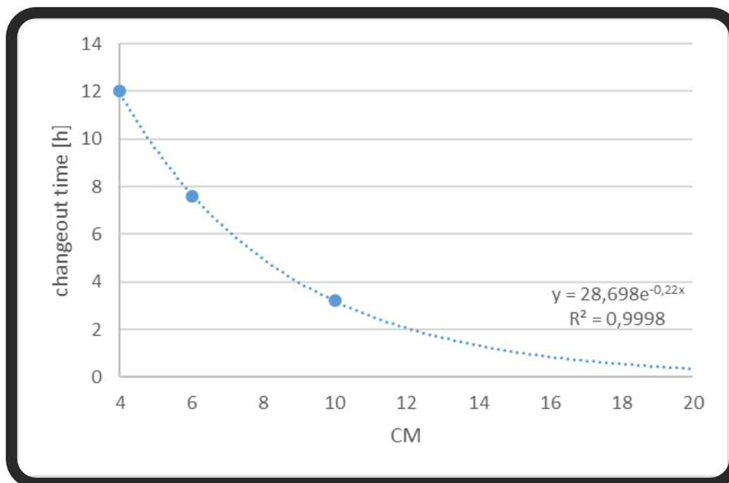
Figure 6-12: LiOH cartridge changeout time estimation
