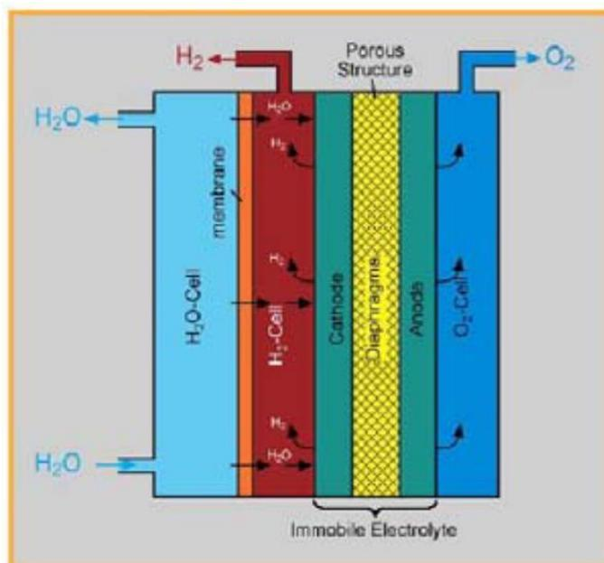
Figure 6-18: ACLS OGA electrolysis principle [88, p. 9]
