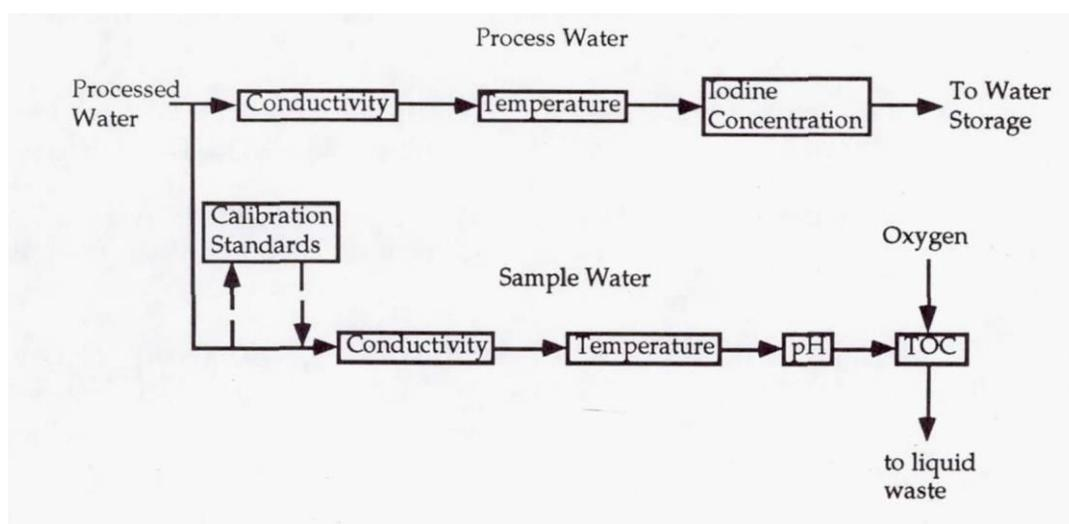
Figure 6-31: Water Quality monitoring process schematic [55, p. 232]
