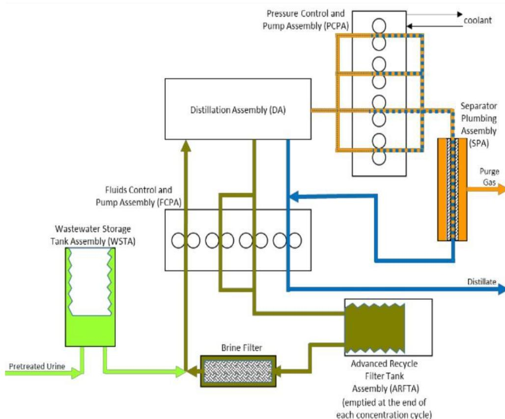
Figure 6-29: Urine processing assembly schematic with ARFTA brine tank [92]
