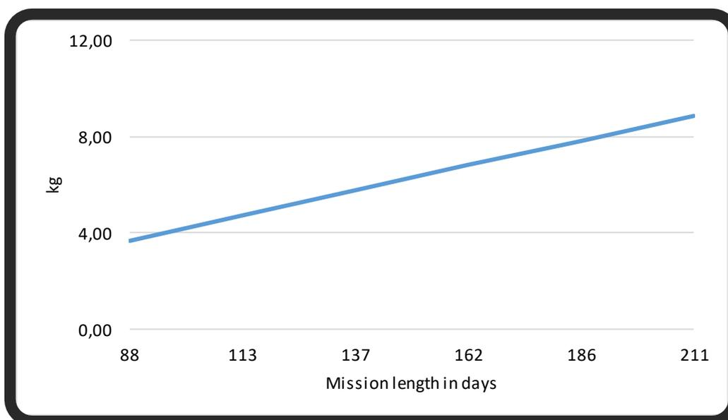
Figure 4-3: O<sub>2</sub> leakage mass over mission length
