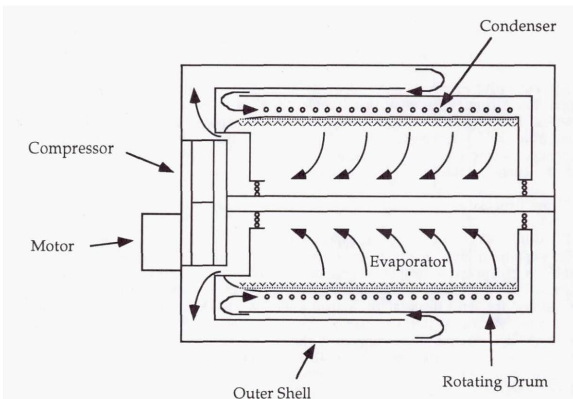
Figure 6-28: Vapor compression distillation schematic [55, p. 229]
