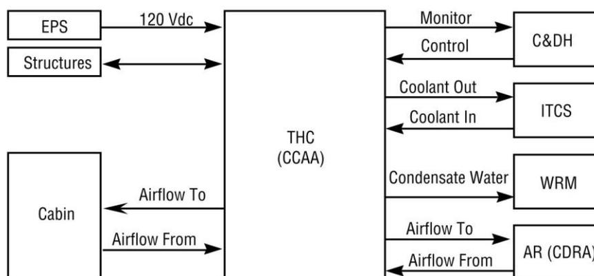
Figure 6-7: THC interface schematic [38, p. 96]
