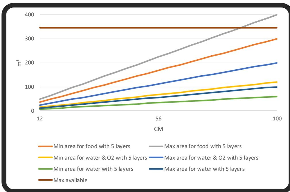
Figure 9-3: Required area for plant growth
