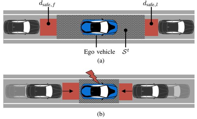
Fig. 1. Visualization of safe free space  $S^t$ : (a) the *safe* free space (shaded area) and the safe distances (red area) of a leading and following vehicle and (b) collisions might be inevitable if the leading vehicle brakes and the following vehicle accelerates.
