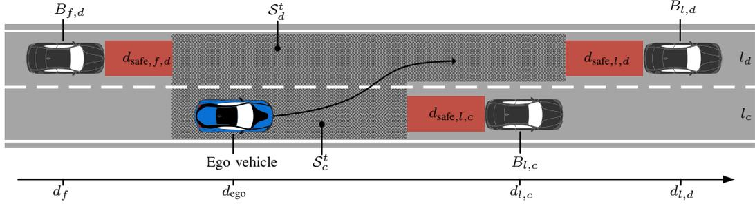
Fig. 2. Visualization of a lane change maneuver: The ego vehicle with position  $d_{ego}$  driving in lane  $l_c$  with a leading vehicle  $B_{l,c}$  wants to change to lane  $l_d$ . This lane contains two vehicles,  $B_{f,d}$  and  $B_{l,d}$ . The safe distances are illustrated in red and the safe free spaces as shaded area.
