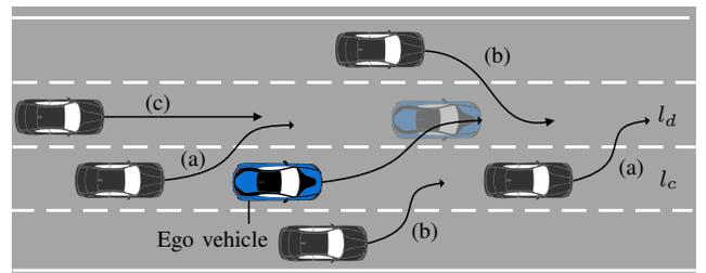
Fig. 4. Possible misbehavior: (a) following or leading vehicles change lanes directly after the ego vehicle, (b) vehicles, neither located on  $l_c$  or  $l_d$ , merge into the safe space, or (c) the following vehicle fully accelerates.
