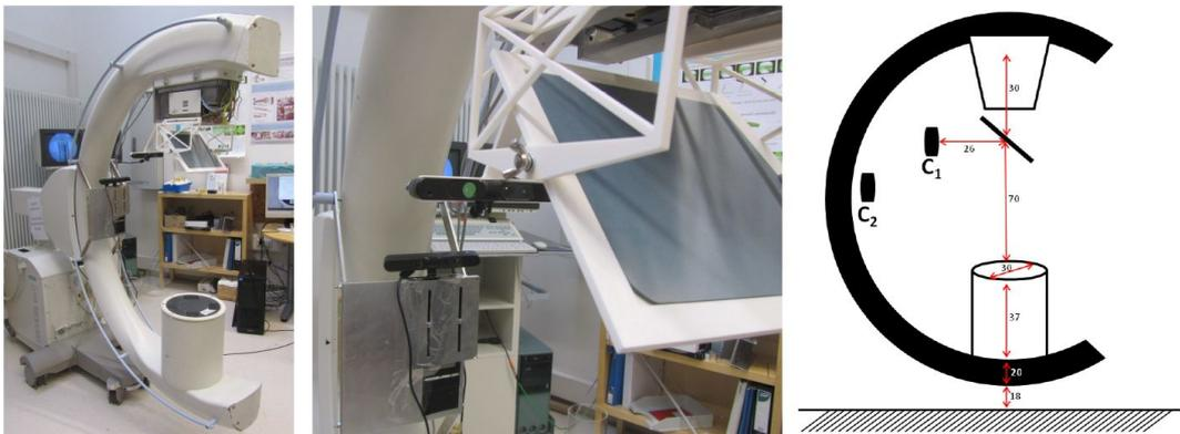
**Fig. 7.1.** (Left, Middle) The setup with the mirror-based RGBD augmented C-arm and an additional RGBD camera, (Right) The setup's sketch including the measured dimensions in centimeters
