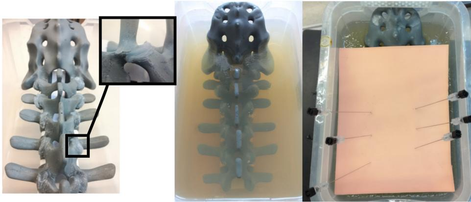
**Fig. 5.18.** Details on the phantom, (Left) Facet Joint simulated by silicone, (Center) Gelatin to simulate soft-tissue, (Right) Fabric cover to simulate skin
