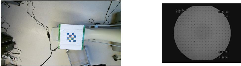
**Fig. 5.7.** Images of the checkerboard used by Wang et al. [173] in the (Left) video and the (Right) X-ray image
