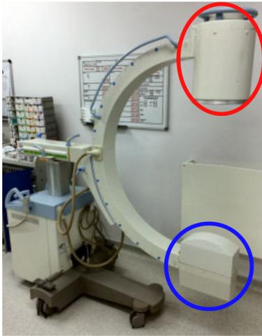
**Fig. 3.5.** C-arm with the image intensifier on the top (red circle) and the X-ray source at the bottom (blue circle), by SteinsplitterBot, distributed under CC BY-SA 4.0 license, Link to Image
