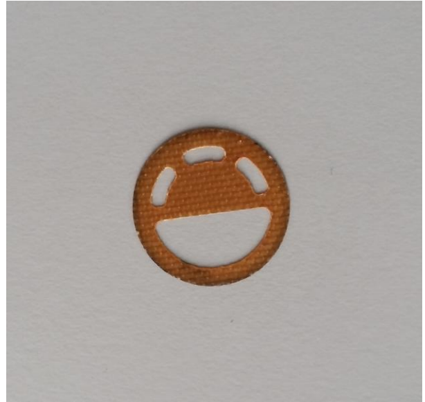
Fig. 6. Nearly all-over cell spacer from a cylindrical Samsung 20700 cell type
