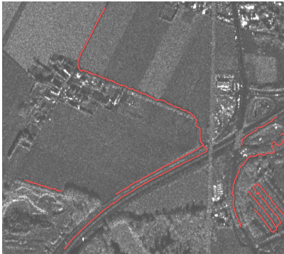
Fig. 6. Extracted roads from one single SAR scene
