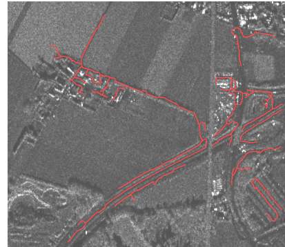
Fig. 8. Extracted roads from two multi-aspect SAR scenes. Global context and the sensor geometry are incorporated during the fusion process.
