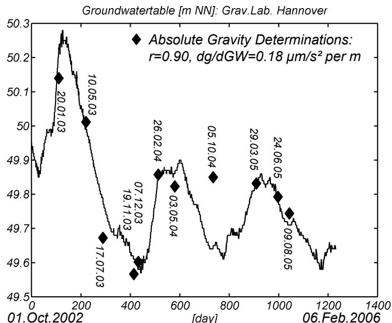
**Figure 1.** Groundwater table at the gravimetry laboratory in Hannover and absolute gravity determinations with FG5-220 since 2003. The two time series are correlated by 90 percent. The derived FG5-220 precision is almost  $\pm 0.01 \mu\text{m/s}^2$ .
