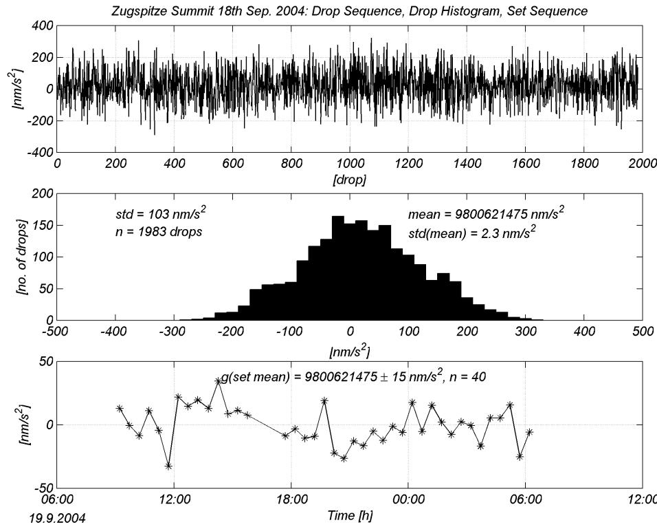
**Figure 5.** Statistical compilation of the station determination ZUG100 (Zugspitze).
