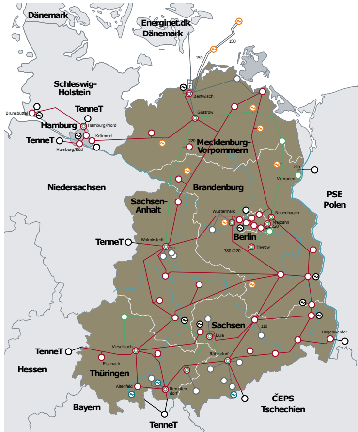
Figure 1.1: Topological overview of the 380/220-kV transmission grid operated by the TSO 50Hertz 1 .
