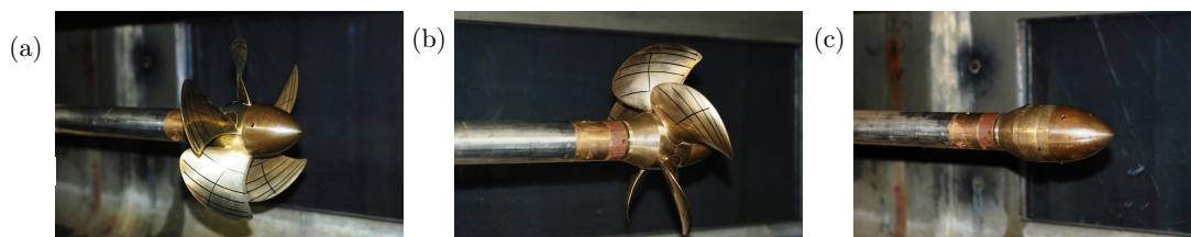
Figure 5.2: Model propeller VP1304 within the cavitation tunnel at SVA, (a) view on suction side, (b) view on pressure side, (c) dummy hub only. Taken from Heinke (2011b).
