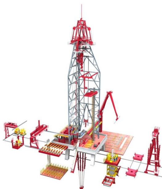
Figure 1-3 A typical conventional topside drilling system 3 (Image: MHWirth AS)
