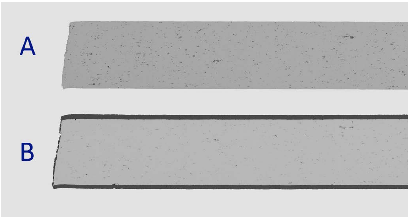
Figure 1: Cross-section of an uncoated (A) and coated (B) U-Mo core. The coating layer shows high homogeneity and follows the surface structure of the U-Mo core well.
