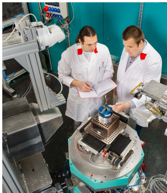
Martin Mühlbauer (left) and Anatoliy Senyshyn used spatially-resolved neutron powder diffraction at STRESS-SPEC in combination with electrochemical measurements and X-ray computed tomography to probe lithium distribution in lithium-ion batteries non-destructively.
