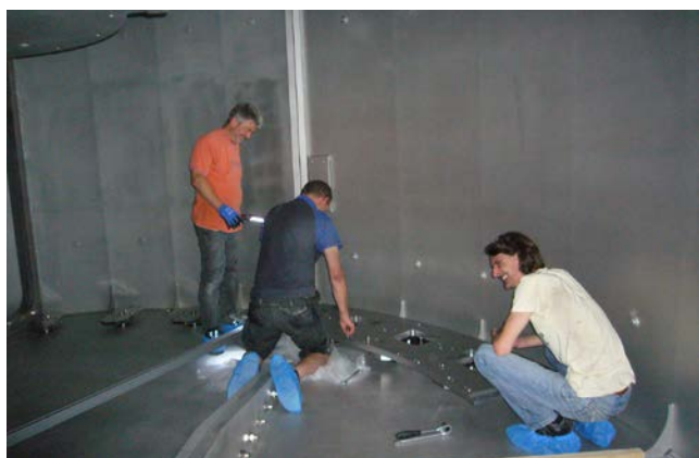
Figure 6: Mounting of the detector benches inside the vacuum chamber of TOPAS.
