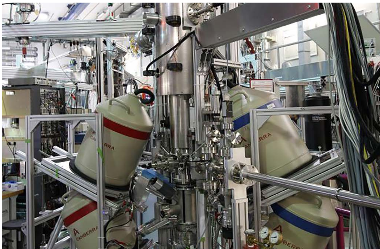
Figure 10: Upgrade of the CDB-spectrometer at NEPMUC with the new optical column and an additional remoderation unit for brightness enhancement. Four high purity germanium detectors pointing to the sample center are used to measure the Doppler-broadening of the positron-electron annihilation line.
