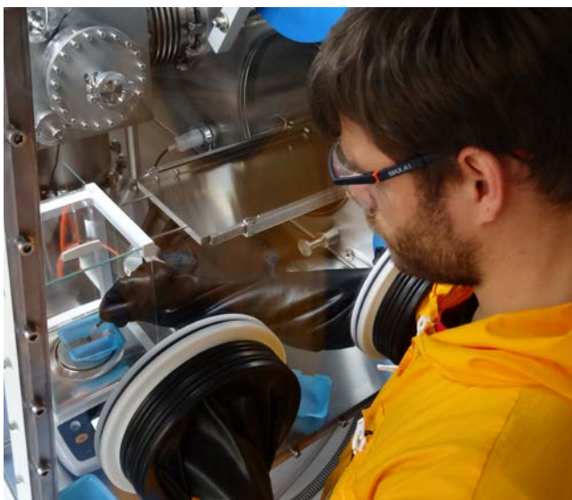
Figure 2: A member of the group handling uranium inside the coating glovebox.
