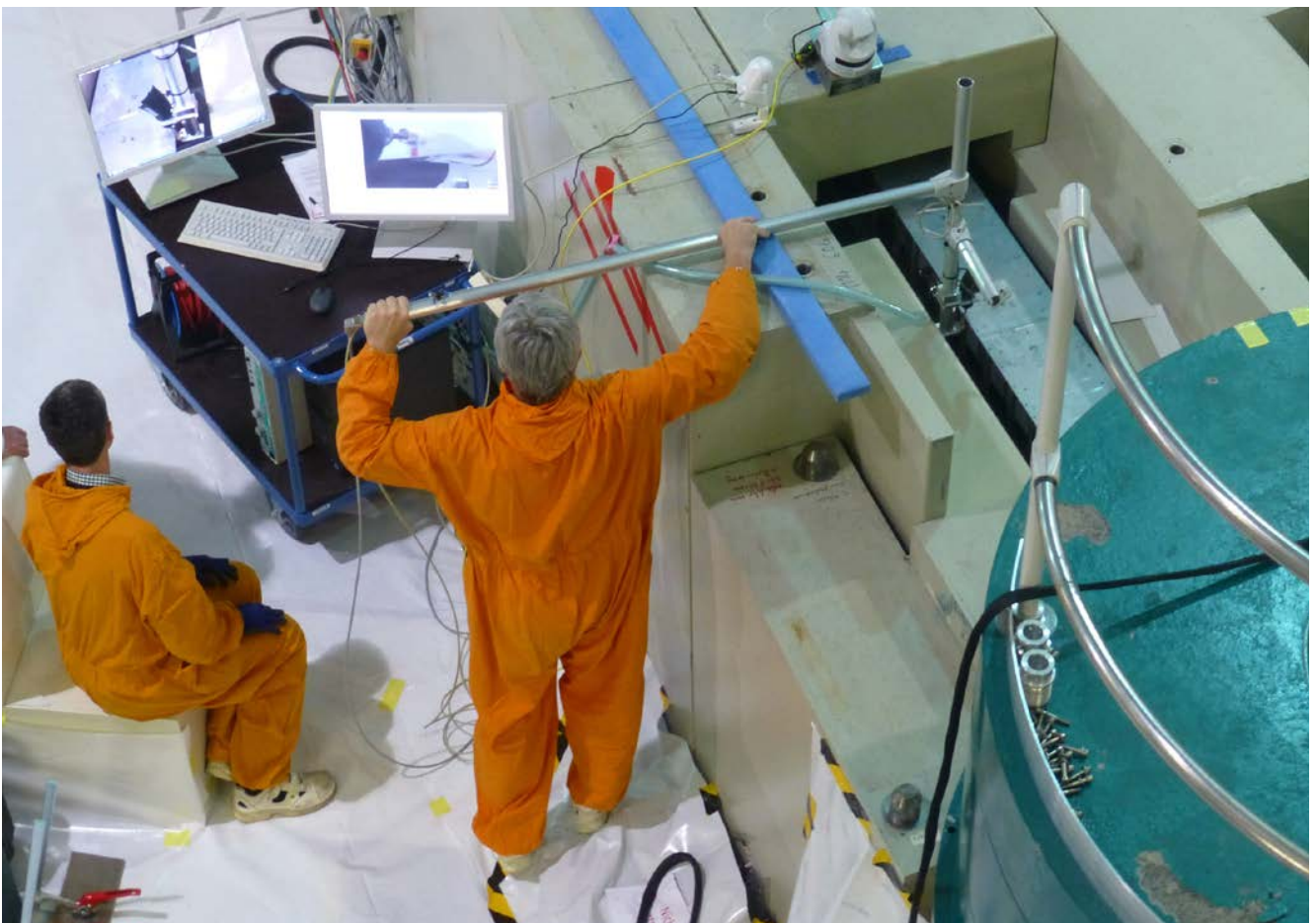
Figure 1: Remote demounting of the magnetic field guide surrounding the neutron guide of the instrument TRISP.
