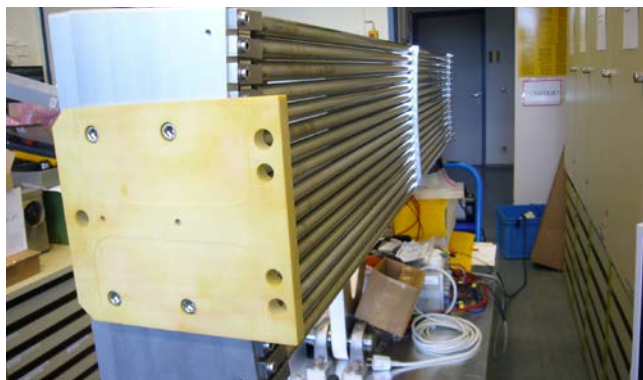
Figure 5: A detector box with sixteen ^3\text{He} tubes in the workshop being prepared for testing.
