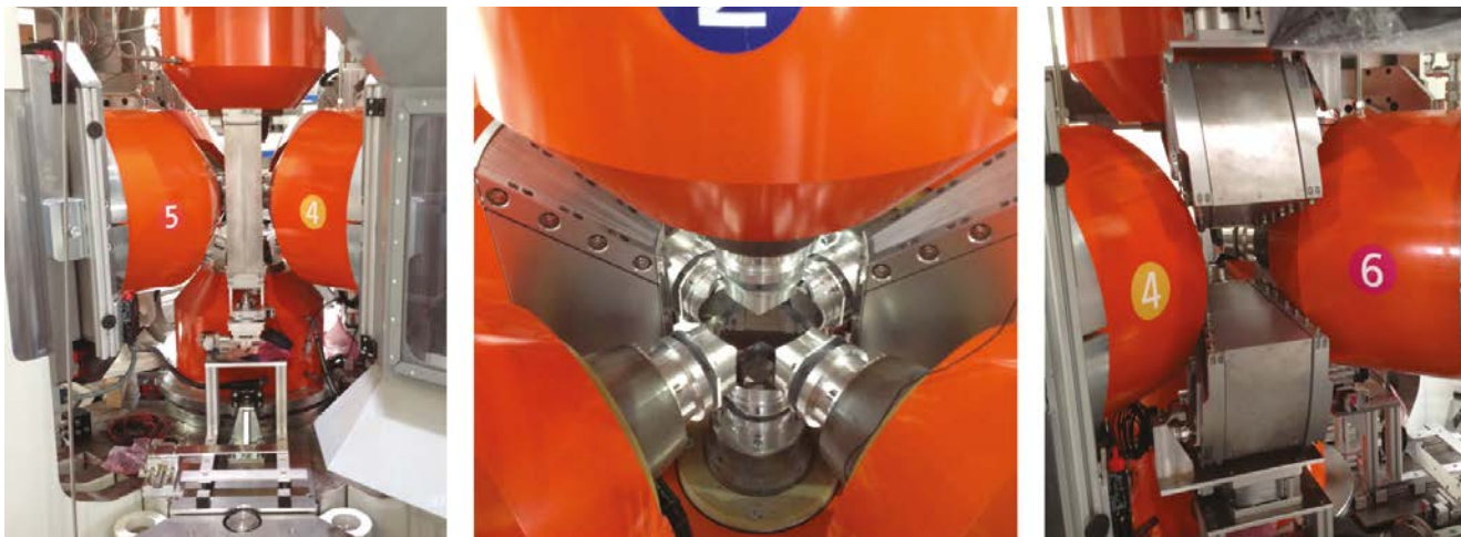
Figure 9: Radial collimators for the 90° detector banks (left) and the backscatter detectors (right). The middle shows the sample position with the primary anvils and the blowout protection.
