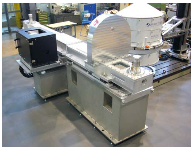
Figure 7: Assembly of the chopper cascade and the neutron analyser in the workshop.
