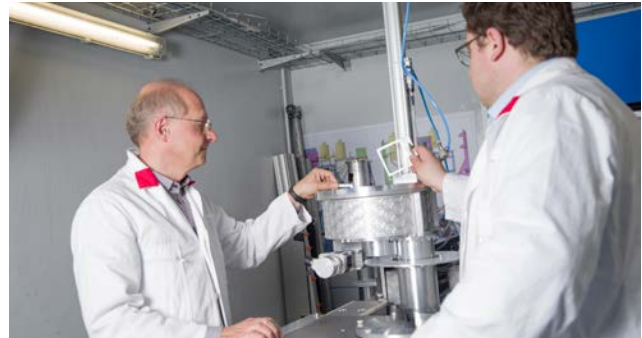
Figure 2: The new PGAA instrument at the MLZ is typically used for the determination of the elemental composition of solid samples, liquids and even gaseous samples.
