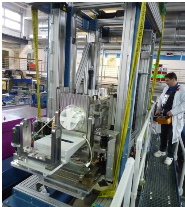
Figure 1: High-precision work with the crane was needed to get the new KWS-3 instrument frame into place.
