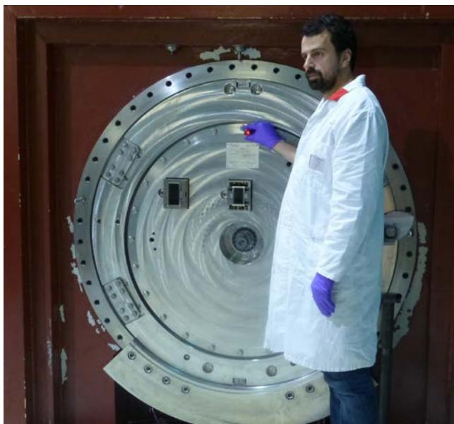
Figure 3: Before closing the beam tube SR5 the beam plug has been adjusted to its theoretical position and the 3 beam line directions have been established employing our laser tracker system.
