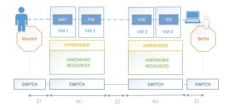
Fig. 1: Service is realized by traversing an ordered set of network functions, in this case Network Address Translation (NAT), firewall (FW), Video Optimization Controller (VOC) and Intrusion Detection System (IDS).
