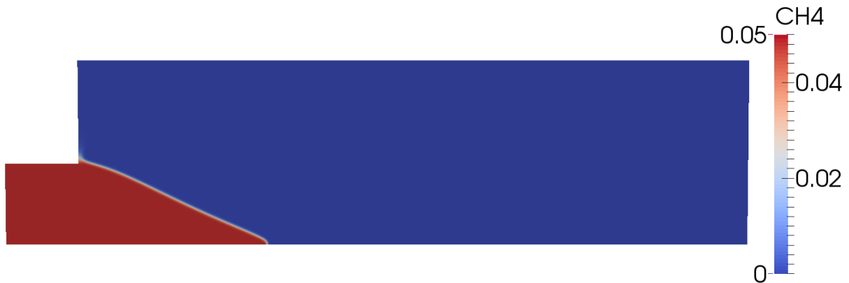
Figure 4.2: Methane profile showing the flame front separating fresh and burnt gas sides.
