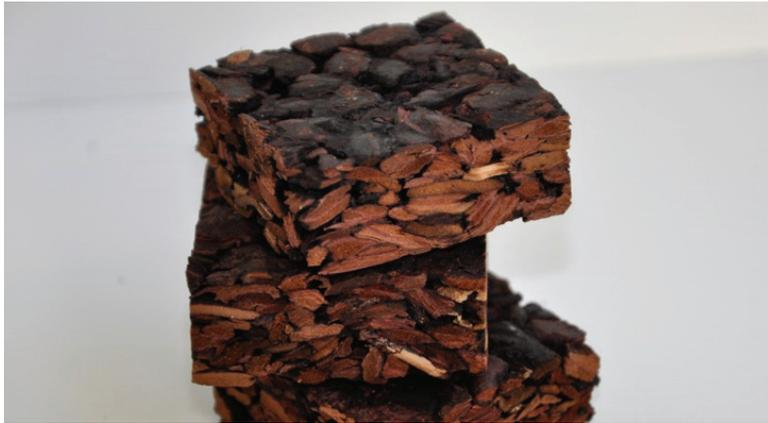
Figure 12. Larch bark-based insulation panel (density 400 kg/m<sup>3</sup>, thickness 20 mm, tannin-hexamine resin, 6 mm ≤ x < 10 mm; Kain et al. 2014).
