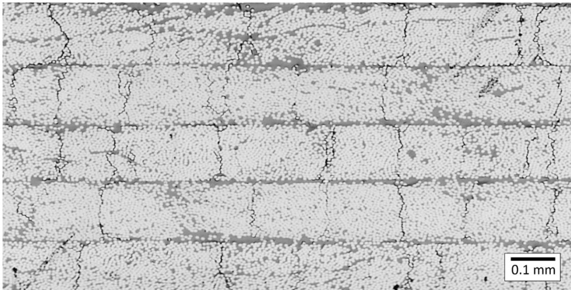
Fig. 3-29: Micrograph of the damage state shortly before ultimate failure of a \pm 45^\circ laminate
