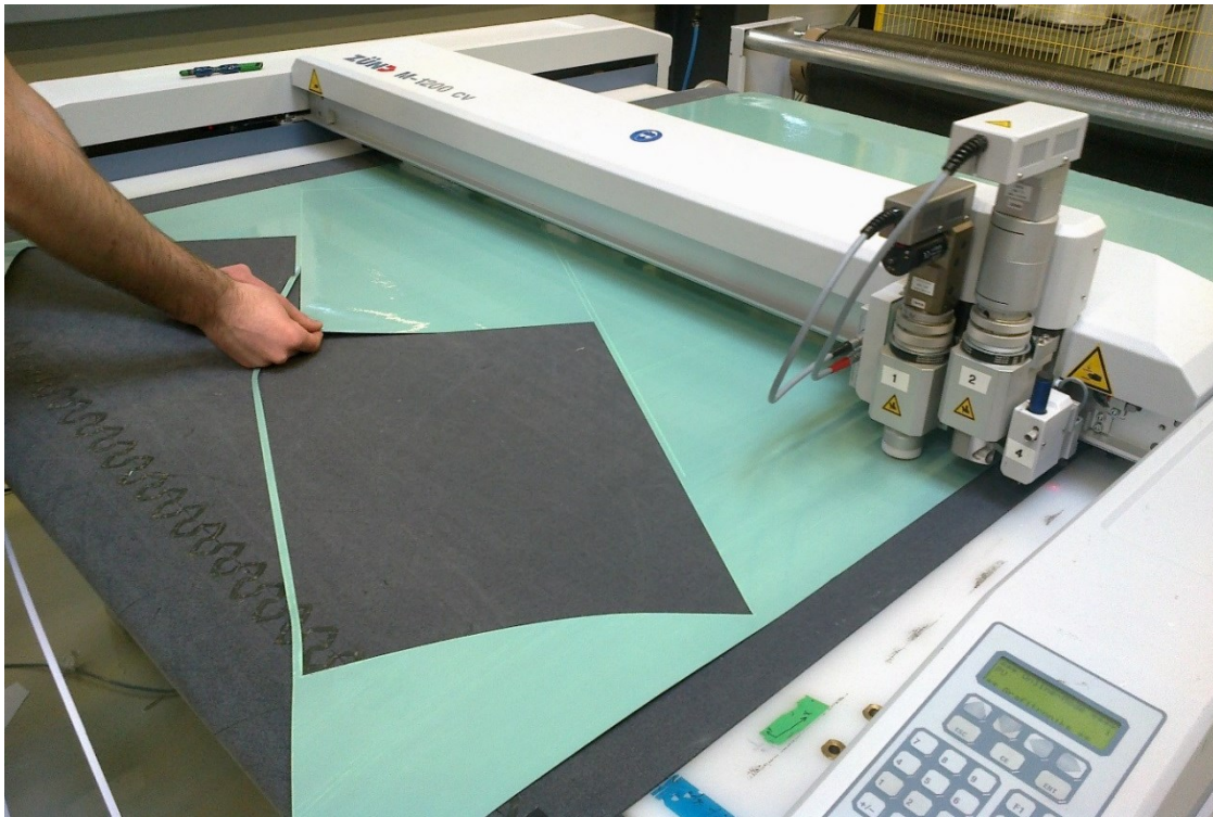
Fig. 3-35: Cutting of the individual layers using a CNC-Cutter
