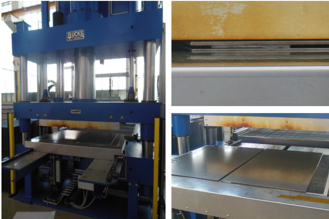
Fig. 3-37: Curing the laminated plates in a Rucks hot press
