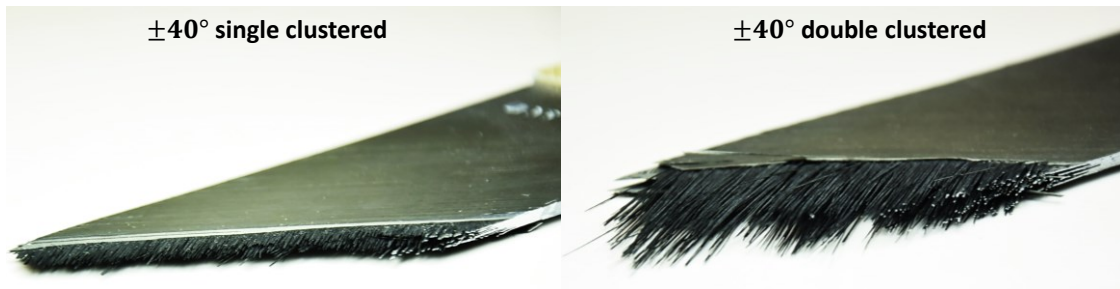
Fig. 4-18: Fracture surface of \pm 40^\circ laminates
