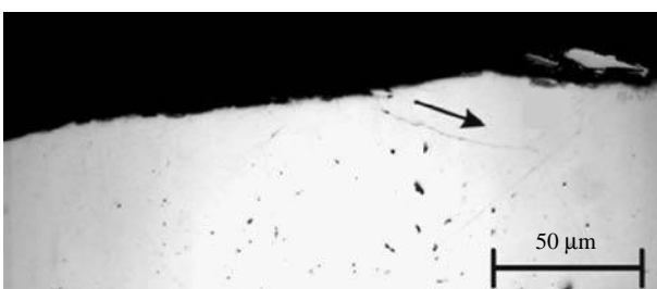
Figure 9 Marine gear: secondary crack in direction to the core (5 mm subsurface)
