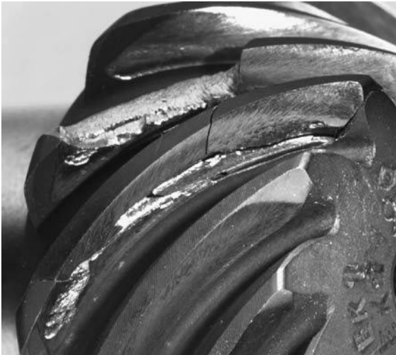
Figure 1 Flank breakage at a test pinion
