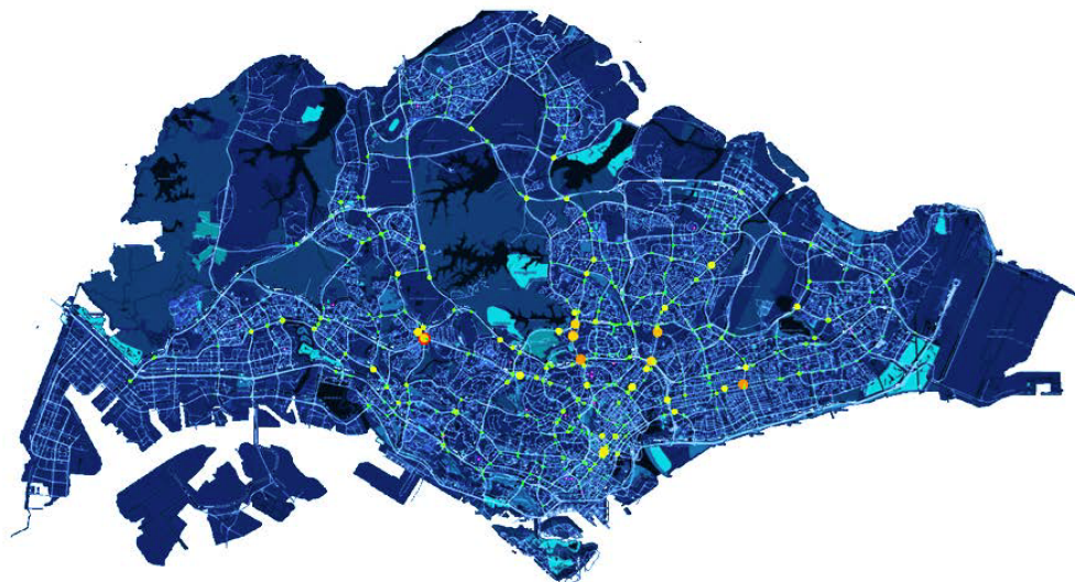
Figure 5.4: Averaged importance value of nodes for a full day. The sensor placement resulting from those values is optimally robust against daily traffic variations.
