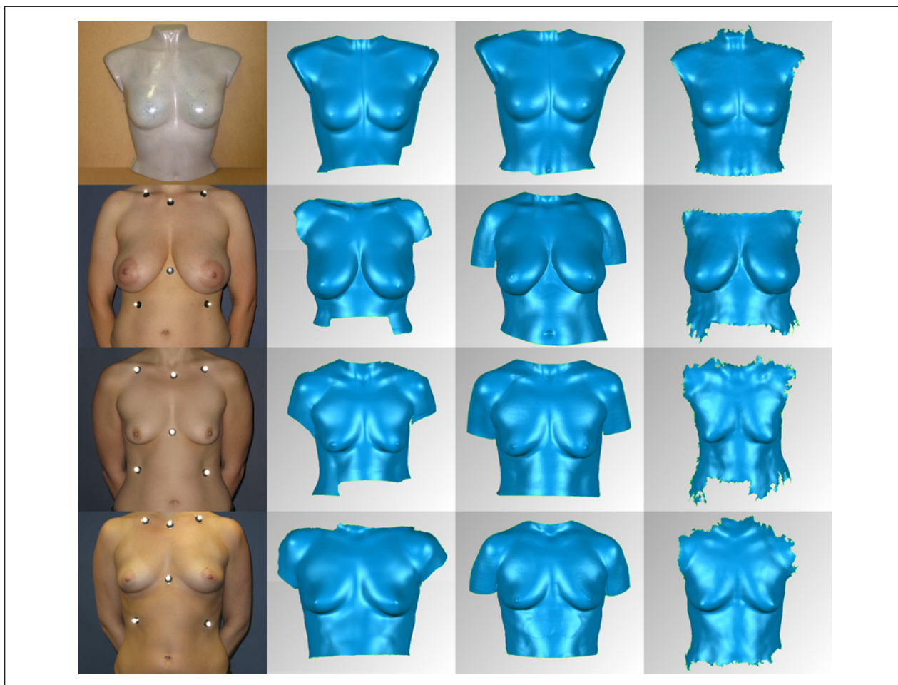
Figure 3. Phantom's and participants' reconstructed surfaces: first column, pictures of the phantom/participants; second column, surfaces reconstructed with SC1; third column, surfaces reconstructed with SC2; fourth column, surfaces reconstructed with SC3.
