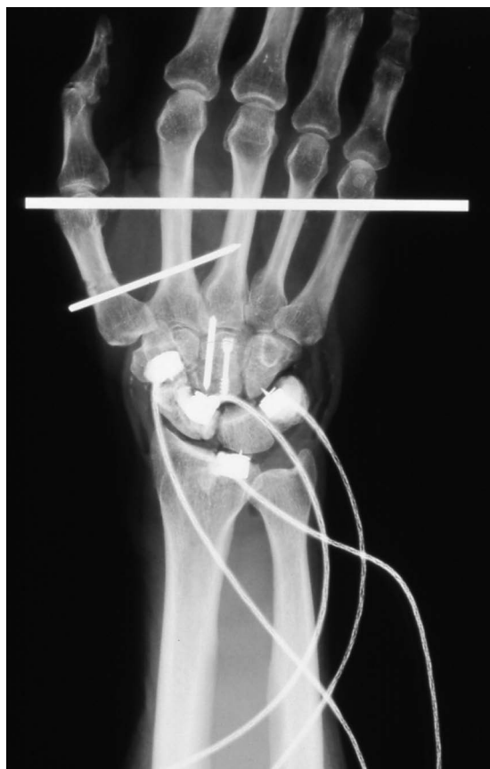
Figure 3. Position of the pressure transmitters seen in the posteroanterior radiograph. Two K-wires were placed to equally distribute load across all metacarpal bones.
