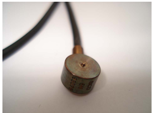
Figure 2. The pressure sensor placed in the intercarpal joints.
