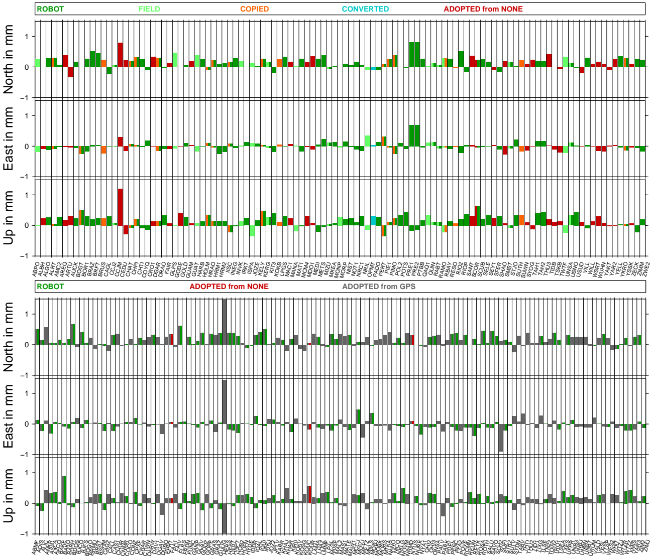
Fig. 6 Change in the repeatability of weekly station coordinates (north, east, and up components) when switching from igs05.atx to igs08.atx phase center corrections for 111 GPS-only (top) and 137 combined GPS/GLONASS stations (bottom). A positive value indicates an improvement of the RMS of the coordinate time series. The colors of the bars refer to different calibration statuses given above the plots. In case the status changed from igs05.atx to igs08.atx (see Sect. 3), the bar is split into two columns (left half referring to igs05.atx, right one to igs08.atx).
