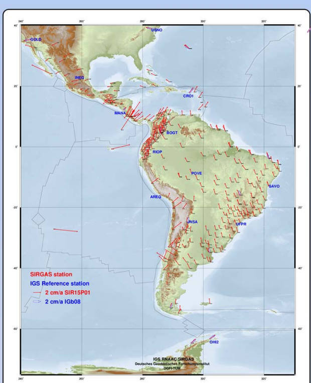
Fig. 4 – Multiyear solution SIR15P01. It covers the time span from 2010.2 to 2015.2, includes 303 stations and refer to the IGB08, epoch 2013.0. Its accuracy is estimated to be \pm 1.8 mm in the horizontal position, \pm 3.5 mm in the vertical position, \pm 1.0 mm/a in the horizontal velocities and \pm 1.2 mm/a in the vertical velocities.
