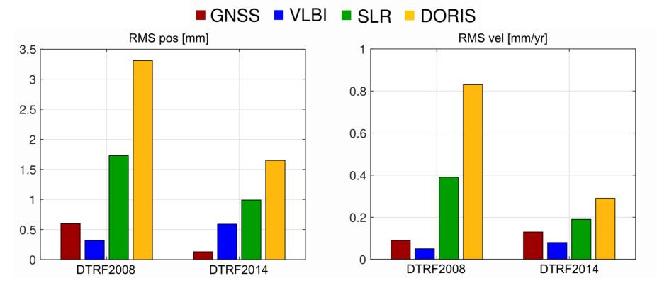
Deformation of network (RMS of Helmert transformation)
