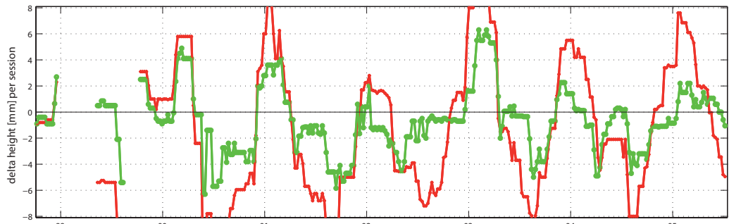
Fig. 1.1.2: Time series of height differences in Tsukuba (Japan): Solutions VMF1 vs. NMF (red) and GMF (green). Displayed are moving medians computed every 7 days for values of 70 days each.
